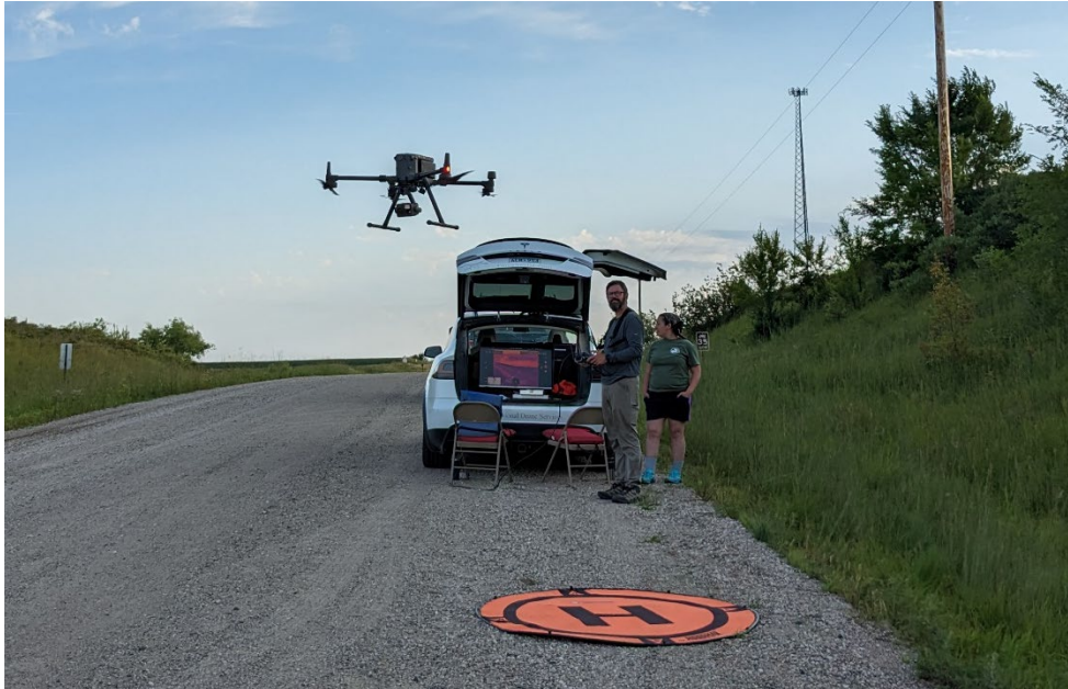
Figure 2. Photograph of UAV launch site for a waterfowl brood survey at Hegg Lake WMA in July 2023 showing typical equipment set-up for 2023 waterfowl pair and brood surveys. The UAV pilot launched the UAV (quadcopter, visible in the air above the road) from a launchpad (orange mat) along a quiet roadside. A monitor in the back of the pilot's vehicle displayed live imagery from the drone camera, with a small map showing the drone's location on an inset screen. During data collection, two researchers watched the monitor from chairs behind the vehicle and coordinated with the pilot to investigate potential waterfowl sightings in thermal imagery and to collect data (counts, species, sex, and age class of waterfowl).
