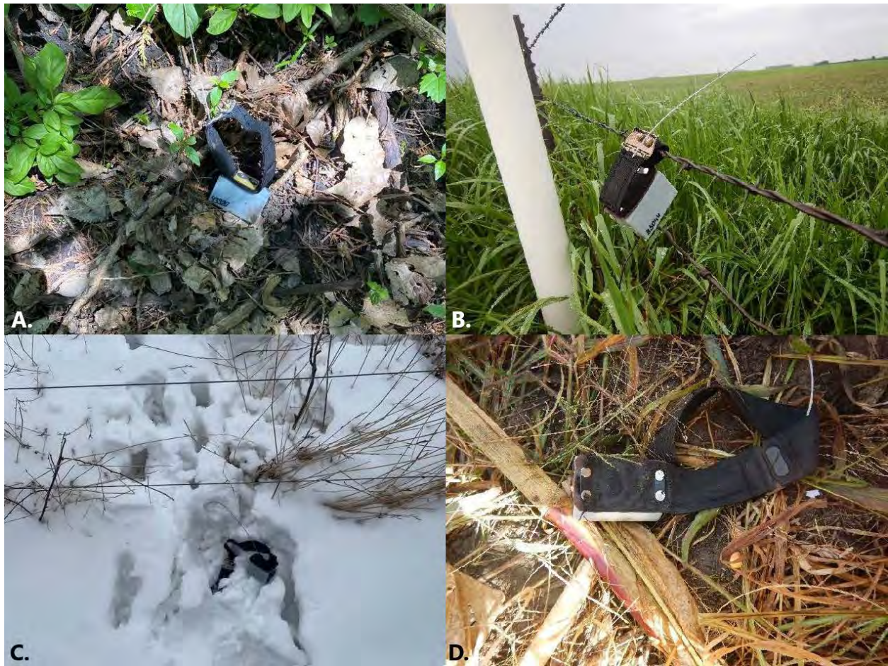
Figure 5. Vectronic Vertex MINI Globalstar expandable GPS collars deployed on white-tailed deer fawns in south central Minnesota, USA in 2021 and 2022. Panels depict: A) a collar that prematurely expanded, B) a collar caught on a fence, C) a collar initially caught on a fence that subsequently broke the expandable band, and D) a collar that got caught on vegetation and the expandable band broke.
