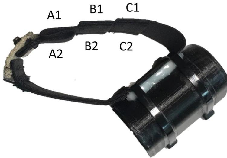
Figure 1. Vectronic Vertex v1.0 collar deployed on white-tailed deer (*Odocoileus virginianus*) fawns at Whitehall Deer Research Facility in Athens, Georgia, USA, during 2018-2019 for testing of experimental designs of Global Positioning System (GPS)-sized expandable radiocollars.
