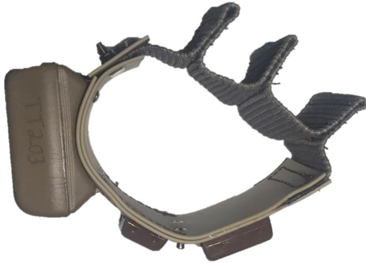
Figure 5. Telonics TGW v2.0 collar deployed on white-tailed deer (*Odocoileus virginianus*) fawns at Whitehall Deer Research Facility in Athens, Georgia, USA, during 2019-2020 for testing of experimental designs of Global Positioning System (GPS)-sized expandable radiocollars.
