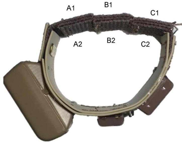
Figure 3. Telonics TGW v1.0 collar deployed on white-tailed deer (*Odocoileus virginianus*) fawns at Whitehall Deer Research Facility in Athens, Georgia, USA, during 2018-2019 for testing of experimental designs of Global Positioning System (GPS)-sized expandable radiocollars.
