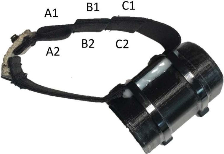
Figure 1. Vectronic Vertex collar deployed on white-tailed deer ( Odocoileus virginianus ) fawns at Whitehall Deer Research Facility in Athens, Georgia, USA, during 2018-2019 for testing of Global Positioning System (GPS)-sized expandable radiocollar designs.
