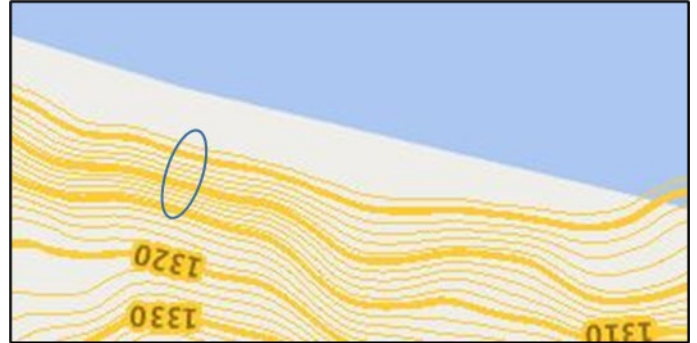
Figure 3. Steepest part of slope is where contour lines are closest.
