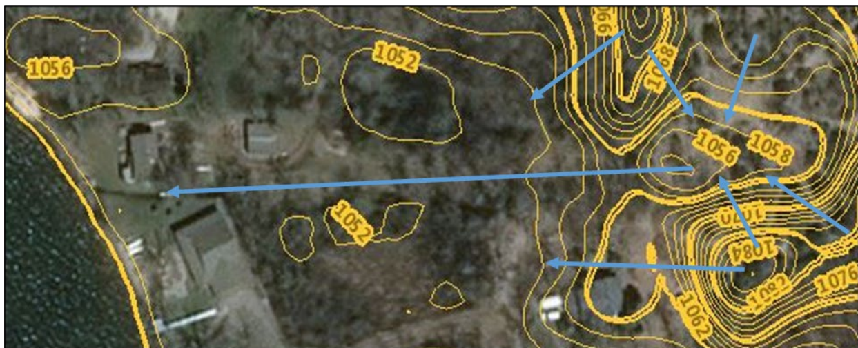
Figure 2. Slope must drain toward the waterbody. Blue lines below indicate water flow based on contours. (Source: MnTOPO)
