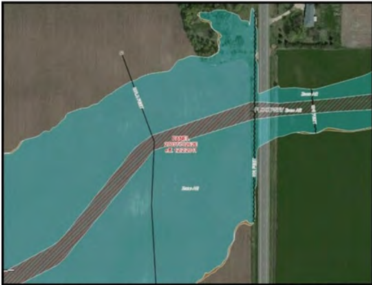
Figure 2: This highlights a scenario where a culvert has concentrated floodwaters, which will further destabilize the stream channel.
