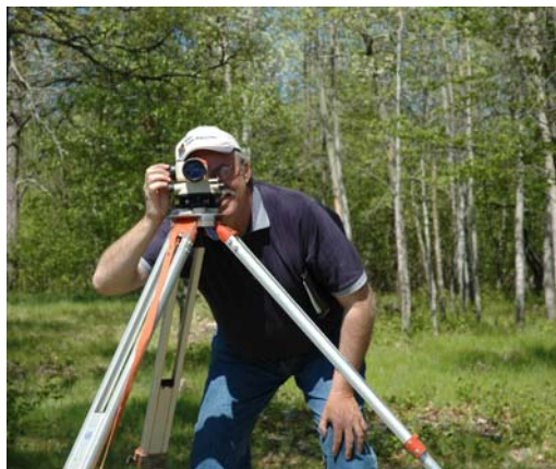
The elevation of each temporary lake gage is surveyed during spring.
