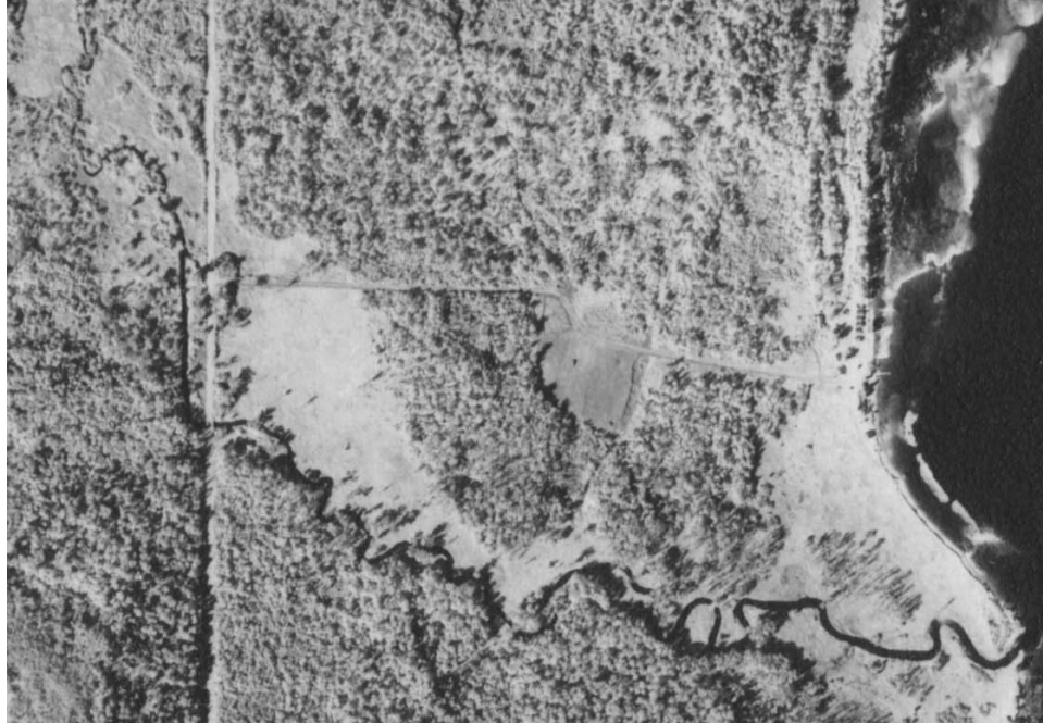
Figure 5.5.16. This 1947 aerial photo was likely taken not long after construction of the road and straight, parallel channel for Moody Creek. Cut off meanders are visible near the tee intersection. (photo from Minnesota Historical Aerial Photographs Online, https://www.lib.umn.edu/apps/mhapo/ )
