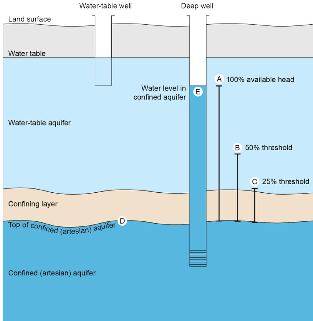
**Figure 3-1** Safe yield thresholds for artesian (confined) aquifers
