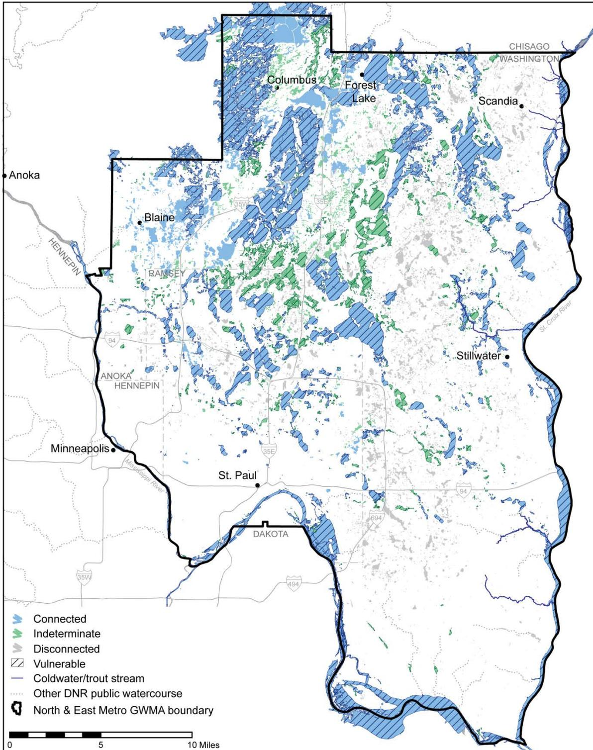
**Figure 2-9** Lake and wetland connection to the regional groundwater system
