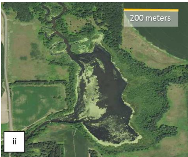
Figure 9. On-site and air photos showing the differences in channel geometry at the 15th Ave NW ds dam site with the impoundment in place in 2017 (i and ii) and with the impoundment removed in 2003 (iii and iv)
