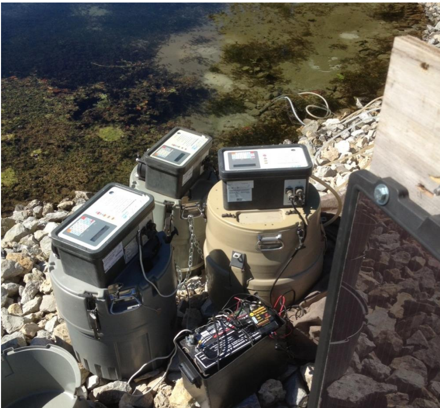
Figure 3. Continuous monitoring using Isco water samplers at the Rostvold spring location
