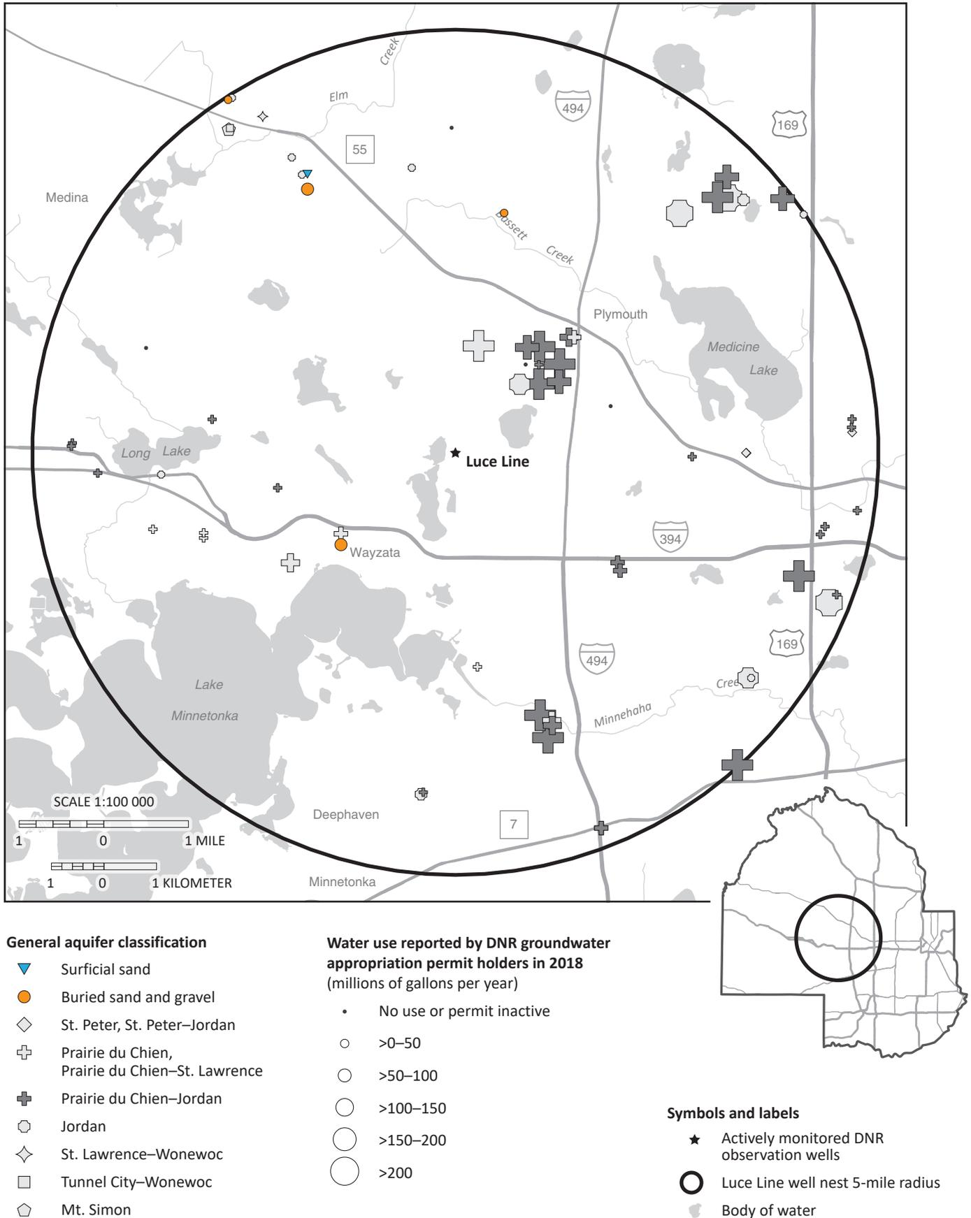
**Figure 24. Groundwater use shown by aquifer within a 5-mile radius of the Luce Line well nest**
