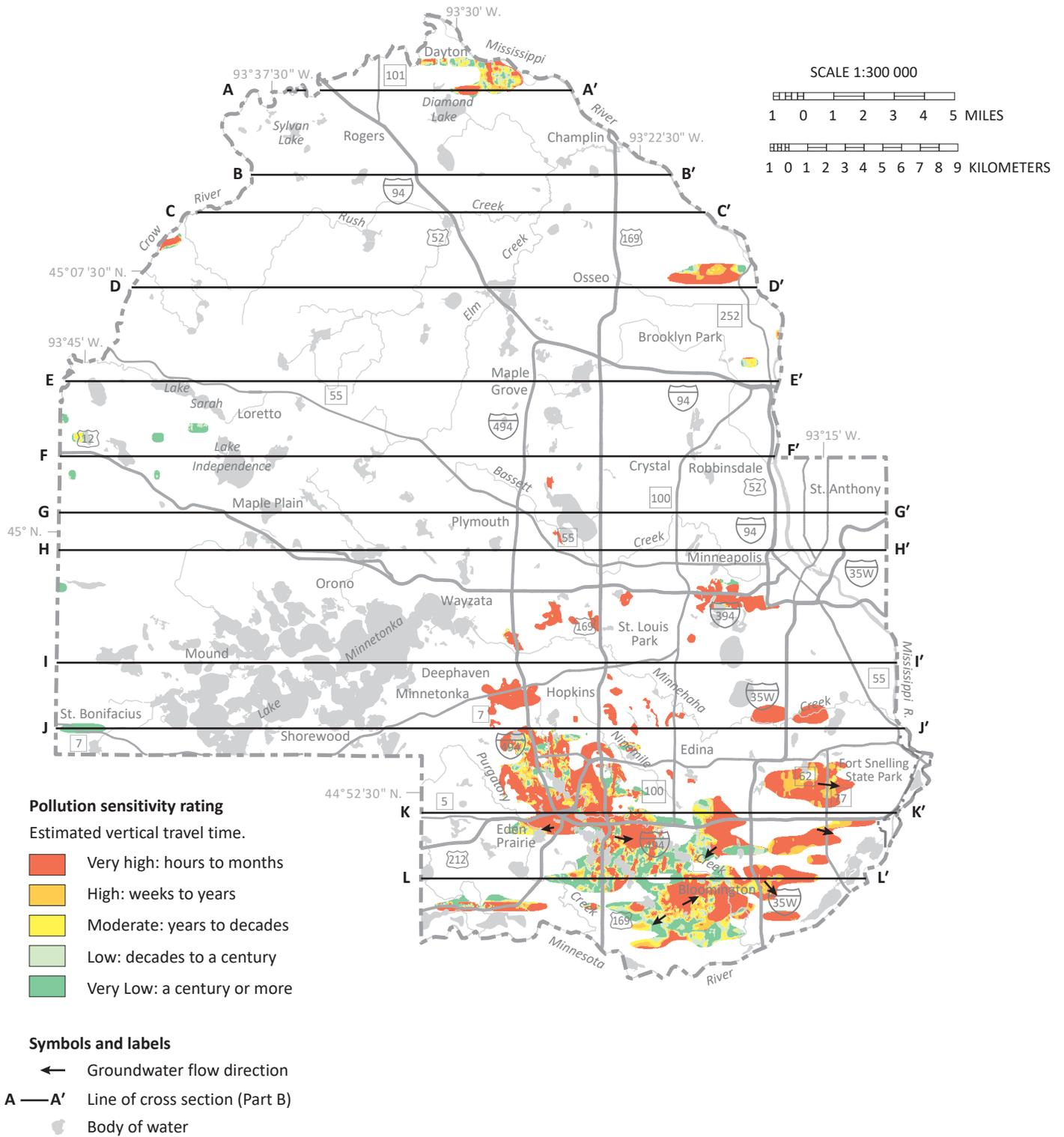
**Figure 38. Pollution sensitivity of the *ti*, *ts1*, and *ms* aquifers and groundwater flow directions**
