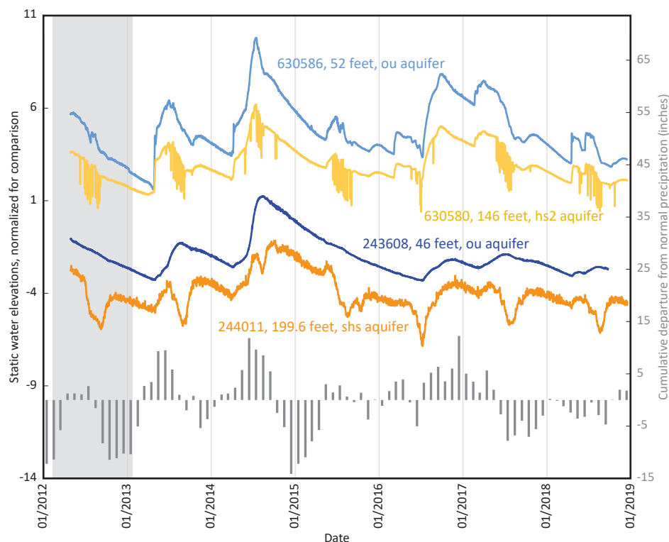
Figure 40. Groundwater hydrograph for two observation well nests in eastern Becker County of responses to large withdrawals
