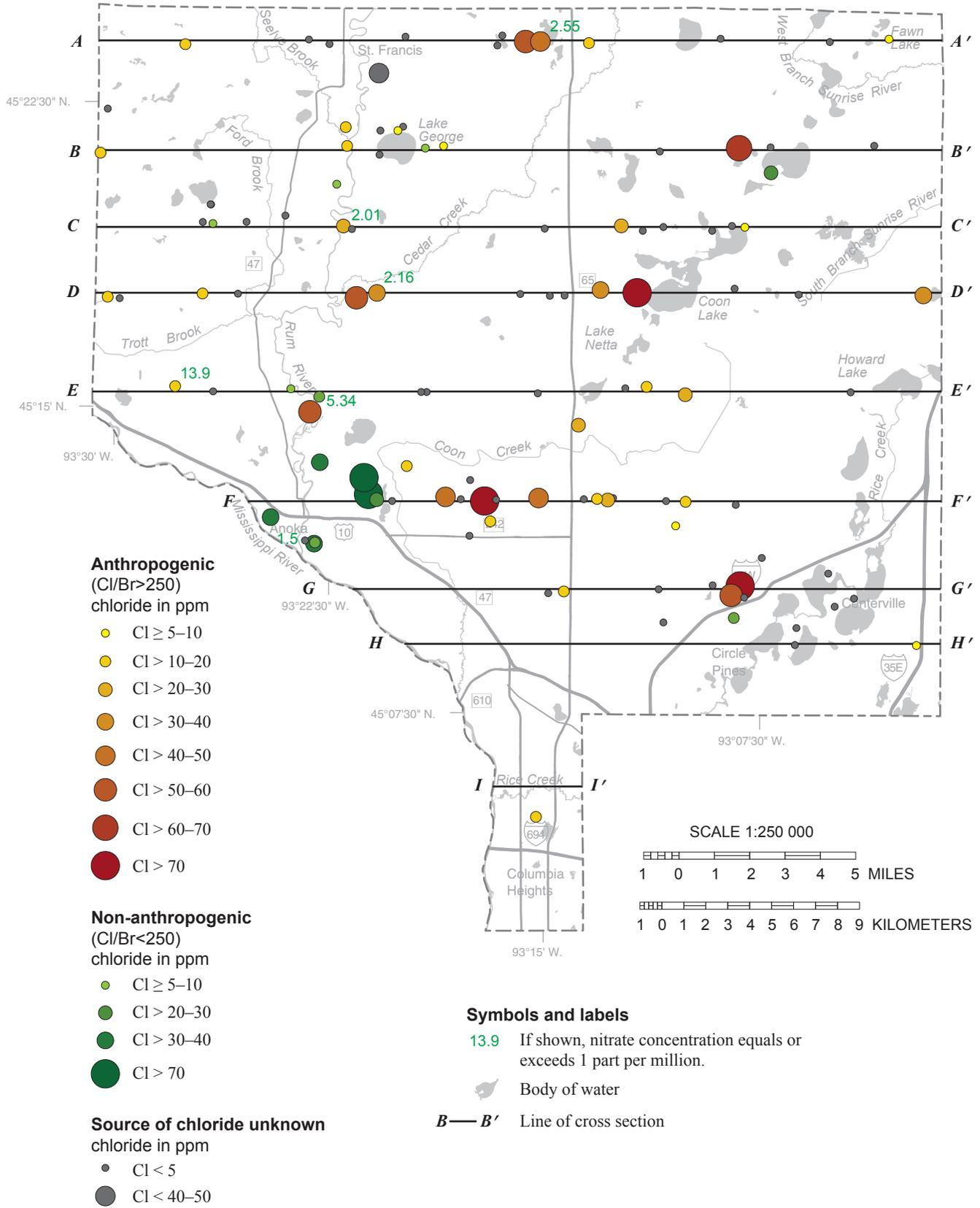
**Figure 19. Elevated chloride and nitrate concentrations from groundwater samples**
