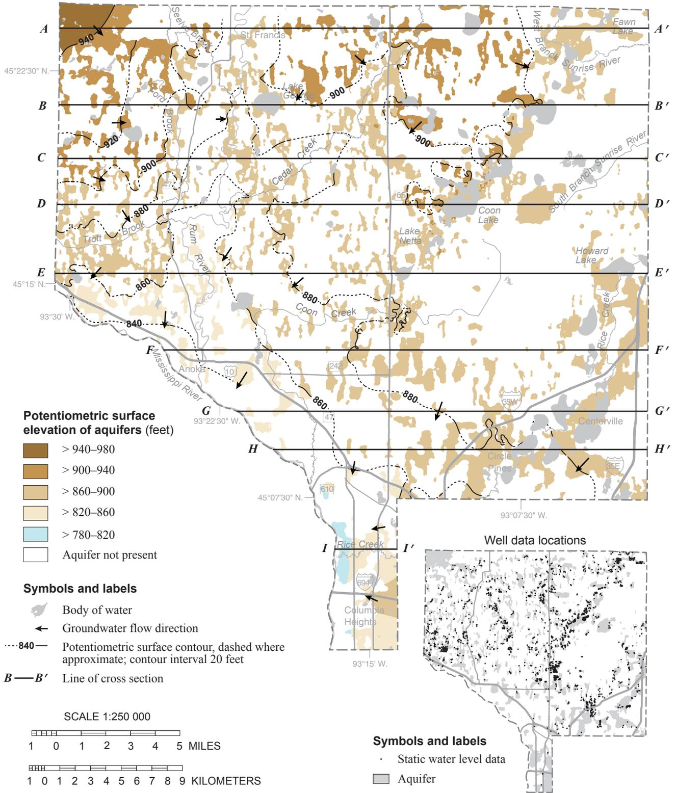
**Figure 7. Potentiometric surface of the sc aquifer**
