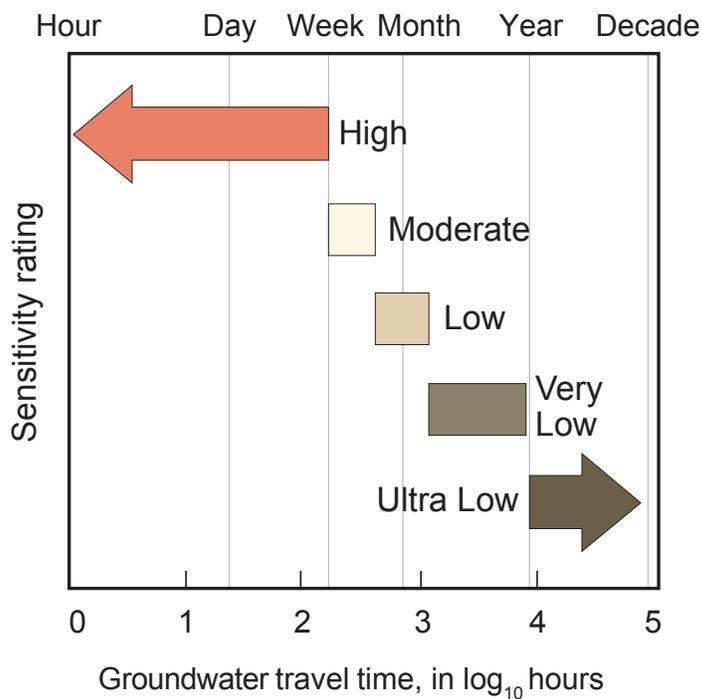
**Figure 21. Geologic sensitivity rating for the near-surface materials**
