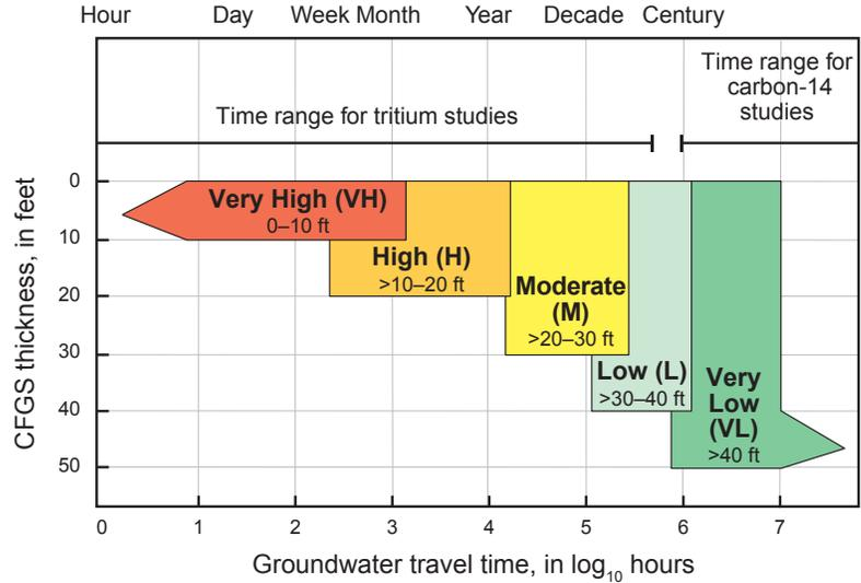
**Figure 23. Geologic sensitivity rating for the buried sand and gravel aquifers and the bedrock surface**
