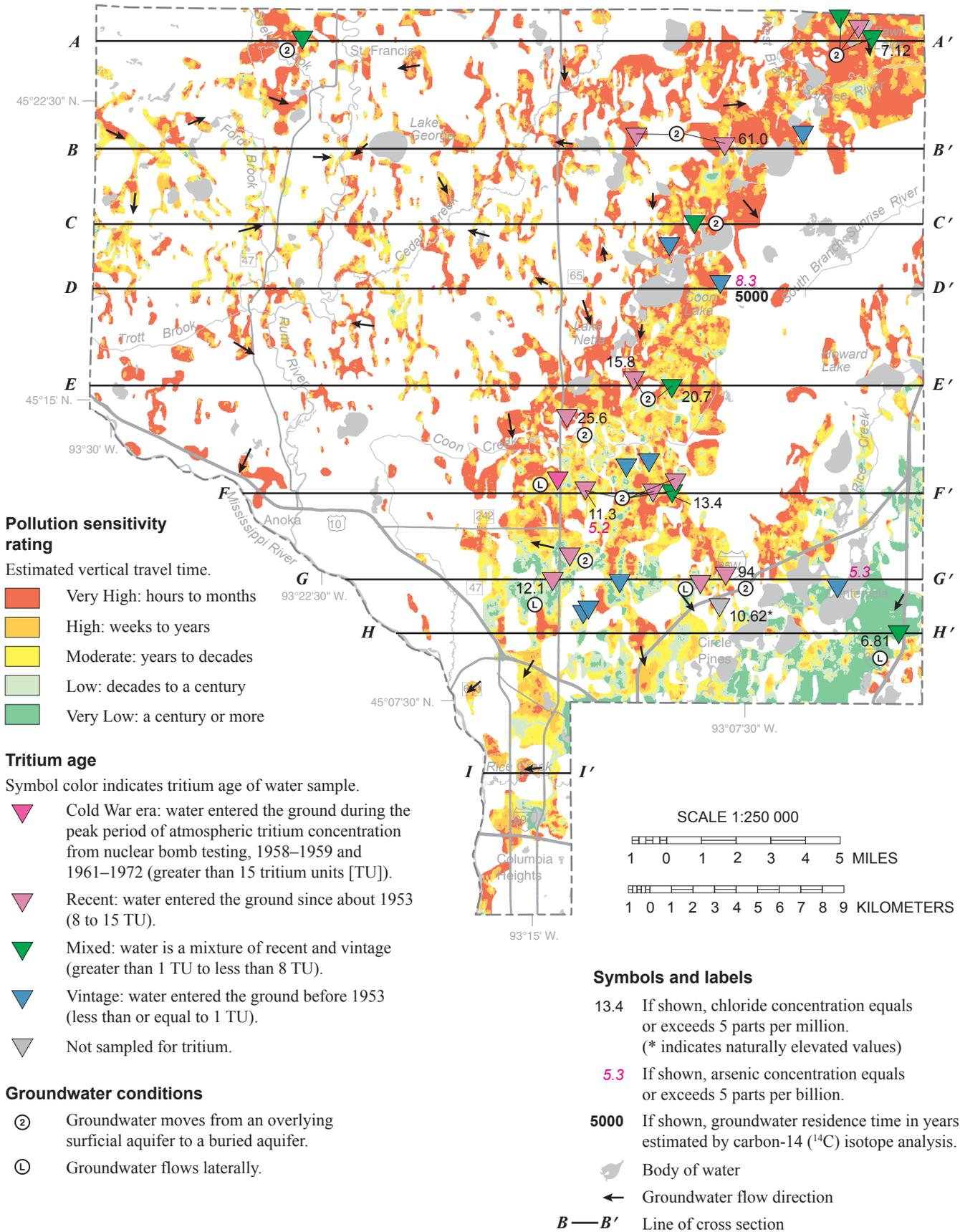
**Figure 25. Pollution sensitivity of the sl aquifer and groundwater flow directions**
