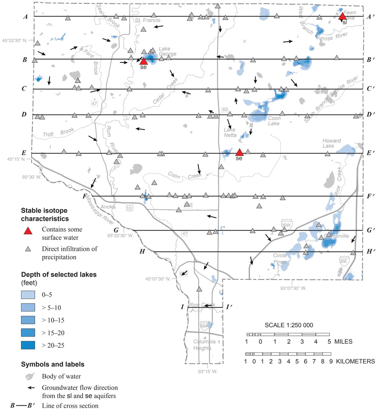
**Figure 17. Stable isotope characteristics of groundwater samples**
