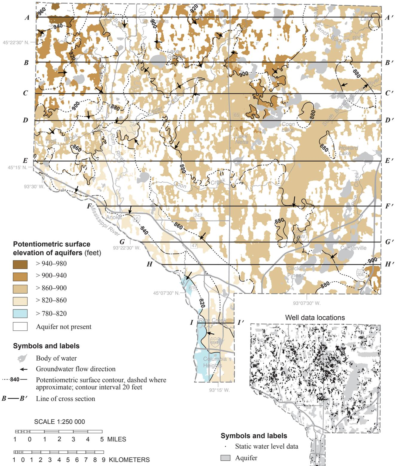
**Figure 8. Potentiometric surface of the se aquifer**
