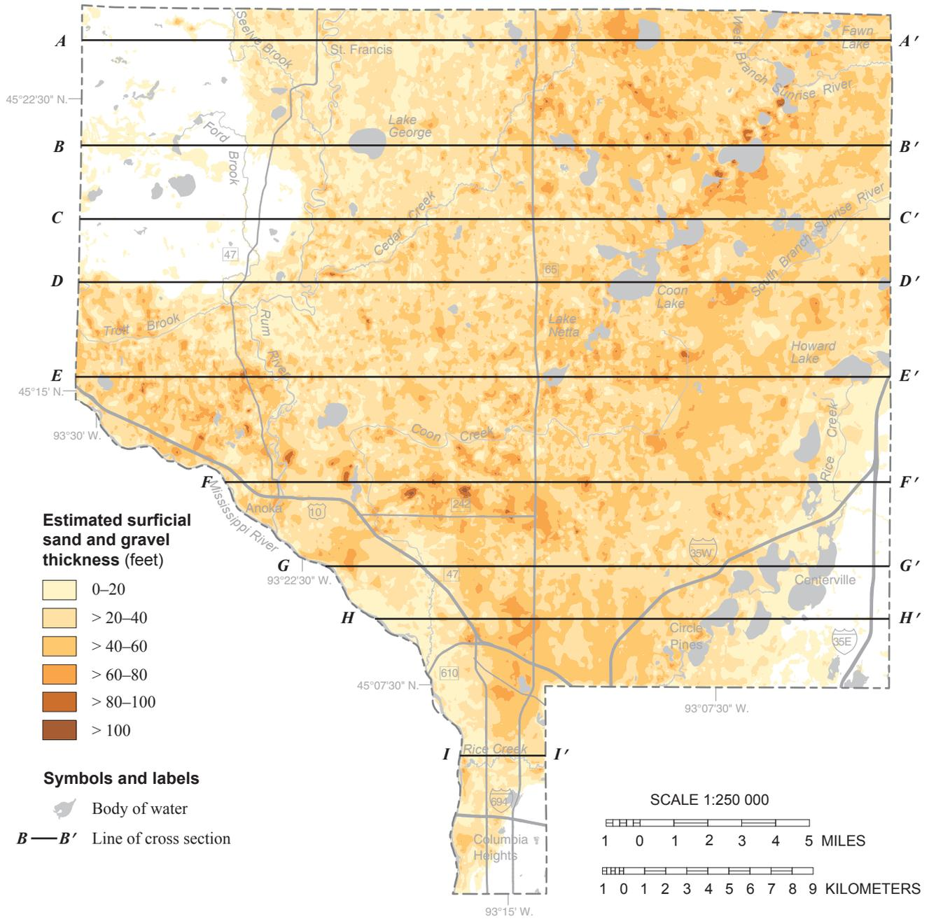
**Figure 2. Surficial sand and gravel thickness**
