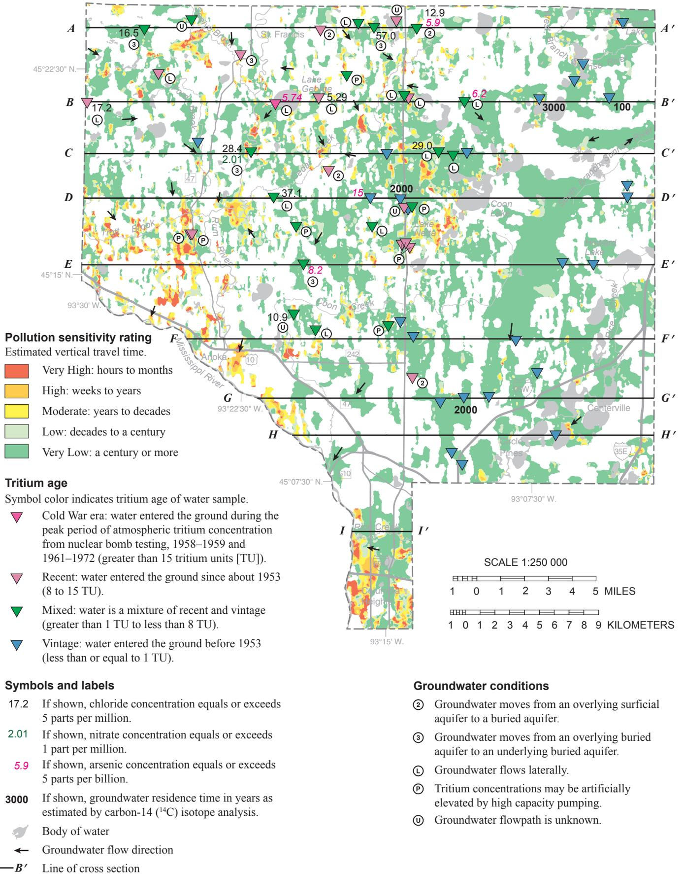
**Figure 27. Pollution sensitivity of the se aquifer and groundwater flow directions**
