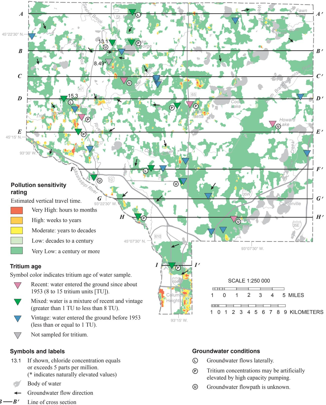
**Figure 28. Pollution sensitivity of the sx aquifer and groundwater flow directions**
