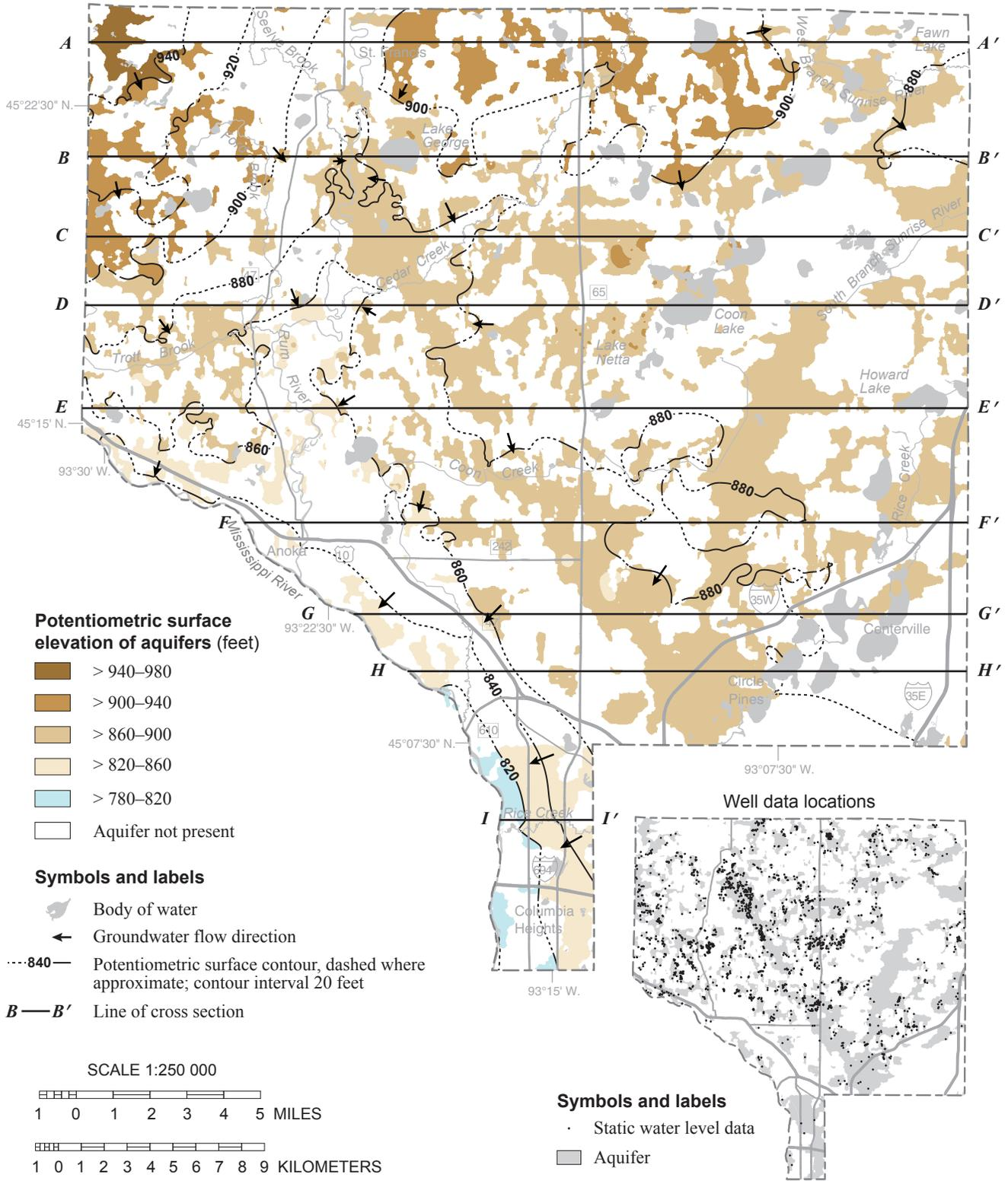
**Figure 9. Potentiometric surface of the sx aquifer**
