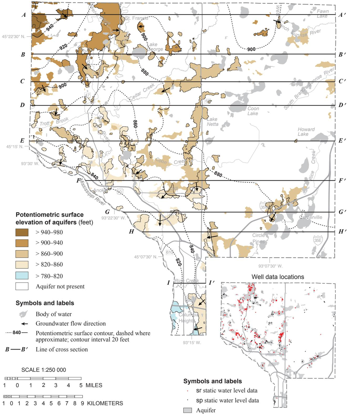
**Figure 10. Potentiometric surface of the sr and sp aquifers**
