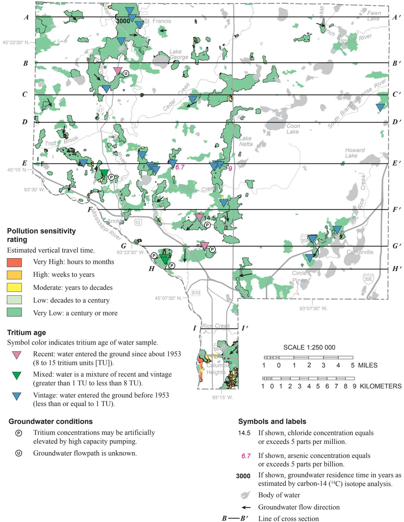
**Figure 29. Pollution sensitivity of the sr and sp aquifers and groundwater flow directions**
