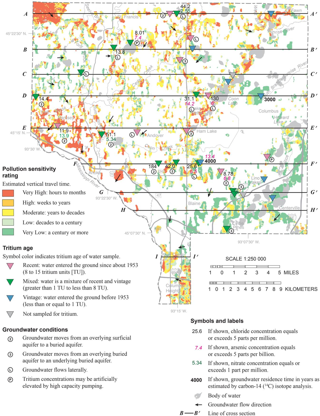
**Figure 26. Pollution sensitivity of the sc aquifer and groundwater flow directions**
