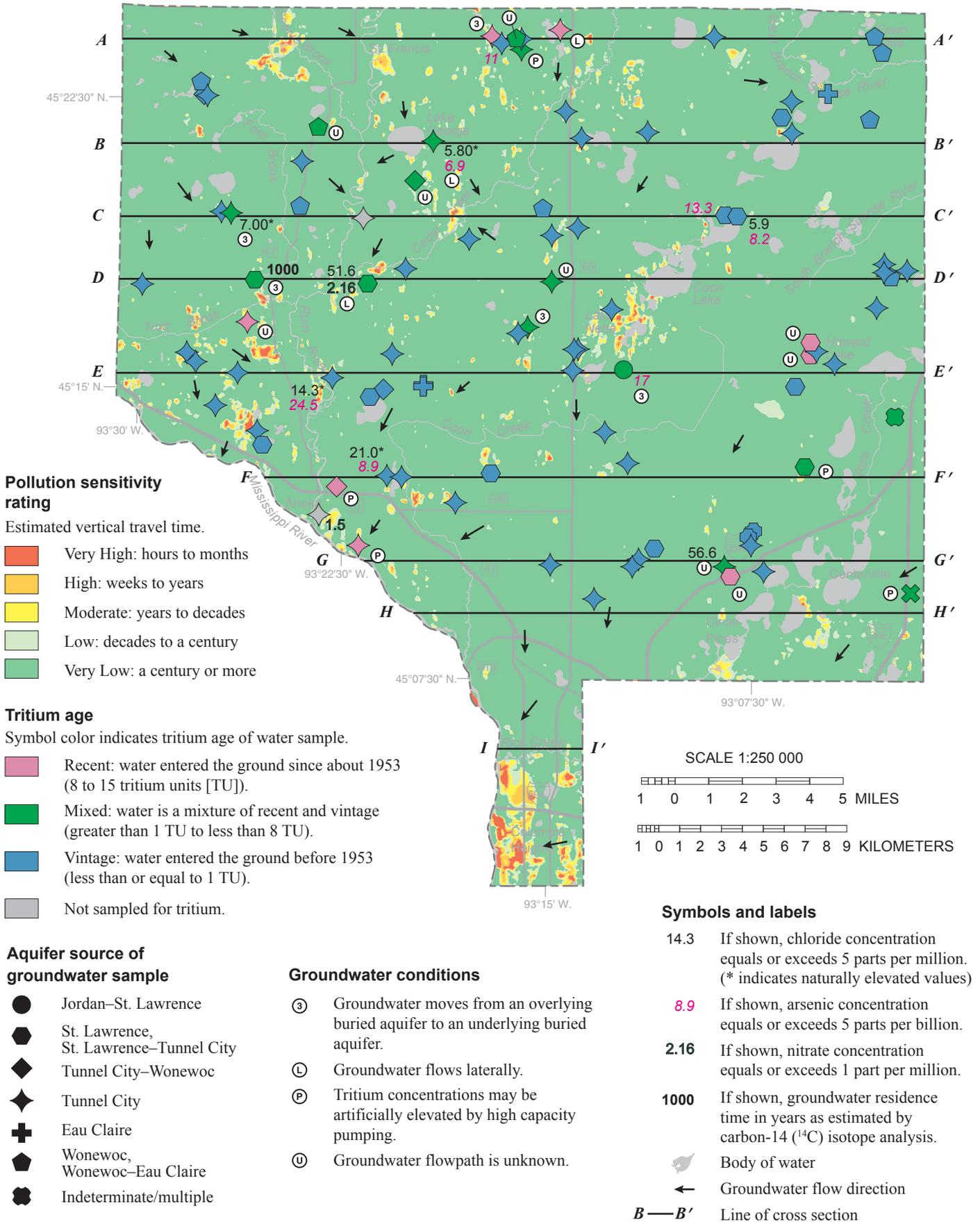
**Figure 30. Pollution sensitivity of the top of bedrock and groundwater flow directions**
