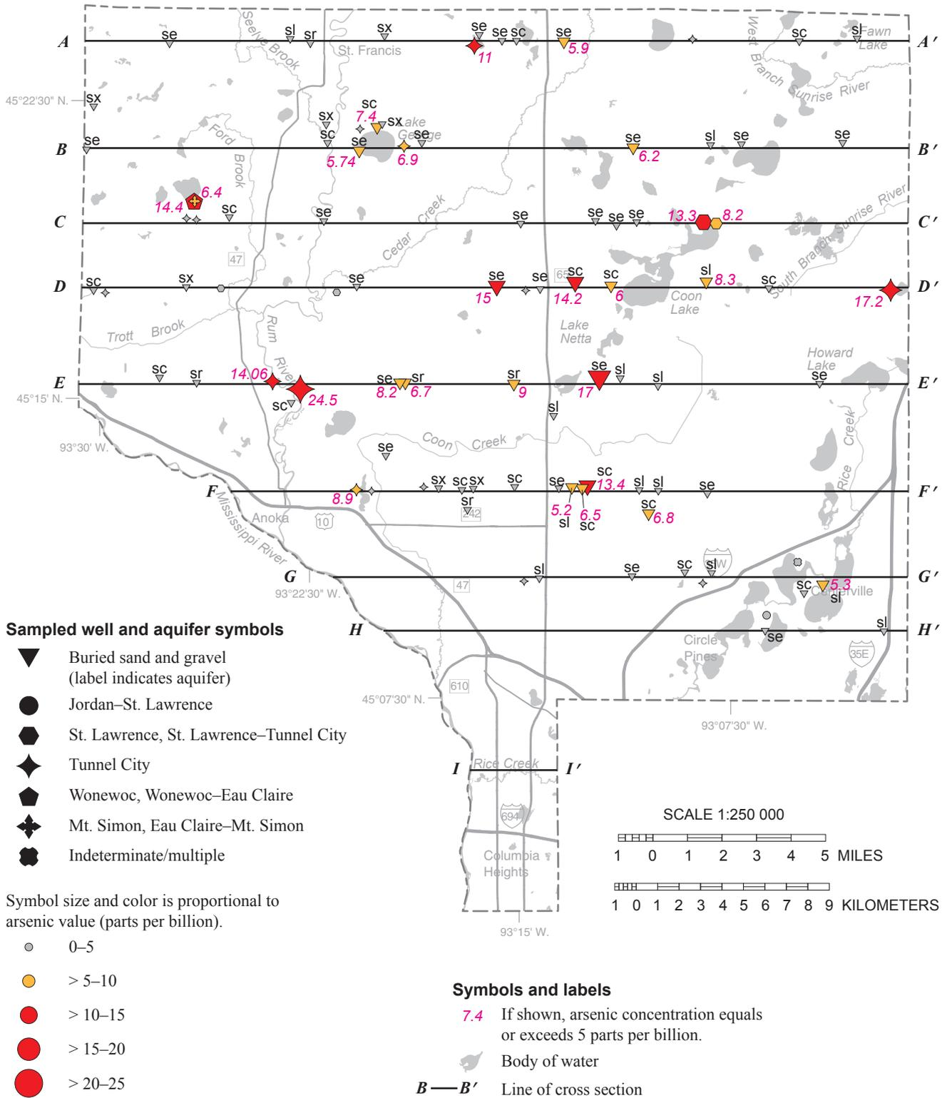
**Figure 20. Arsenic values from buried sand and bedrock aquifers**
