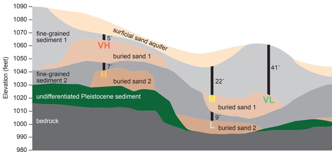
**Figure 24. Cross section showing examples of pollution sensitivity ratings**
