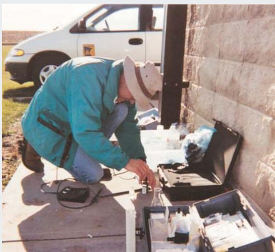
DNR Waters conducts some tests on water samples in the field after drawing a ground-water sample from a well. This hydrologist is testing water from a well near Plainview.
