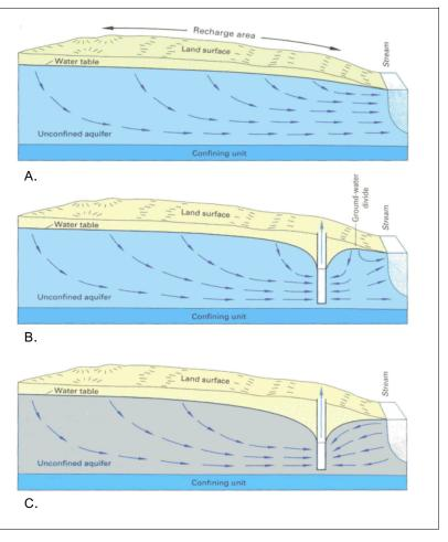
Figure 13. A. Normal streamflow, B. stream capture, and C. stream interception (USGS Circular 1139)
