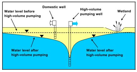
Figure 12. Water supply interference
