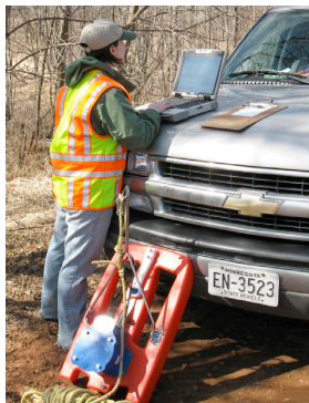
DNR hydrologist prepares to collect stream flow data with the orange Acoustic Doppler Profiler.
