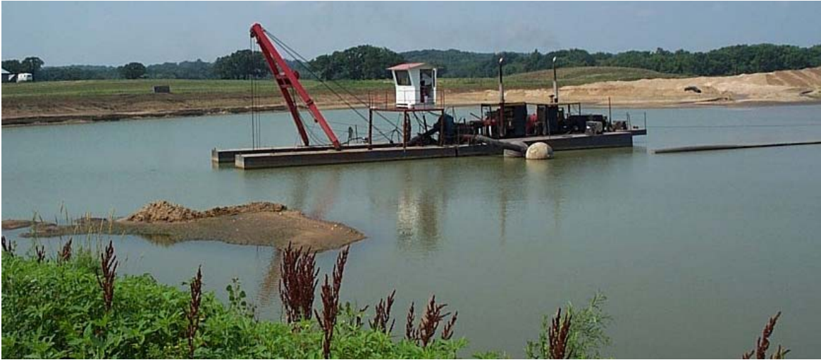
Figure 5. Donovan pit mining with a hydraulic dredge.
