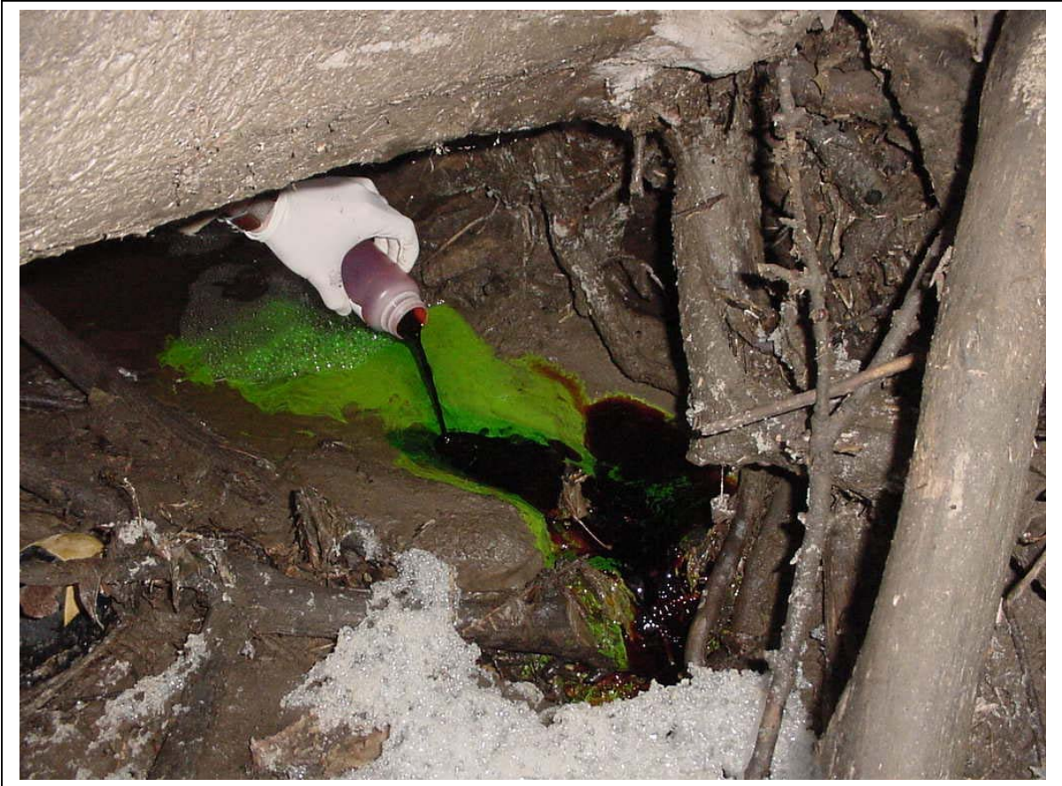
Figure 5. Introducing dye into the stream of water.
