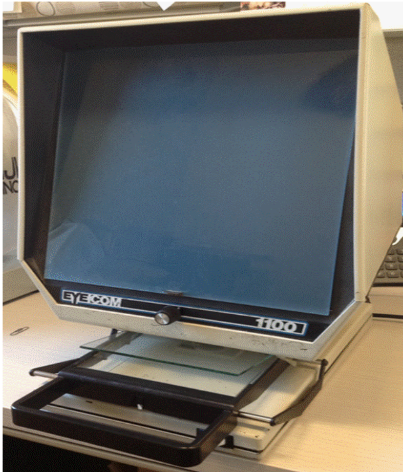
Figure 18. Microfiche reader used to magnify scale images.
