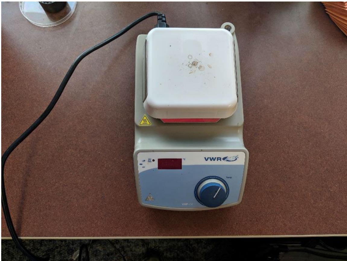
Figure 6. Hot plate used to brown otoliths.
