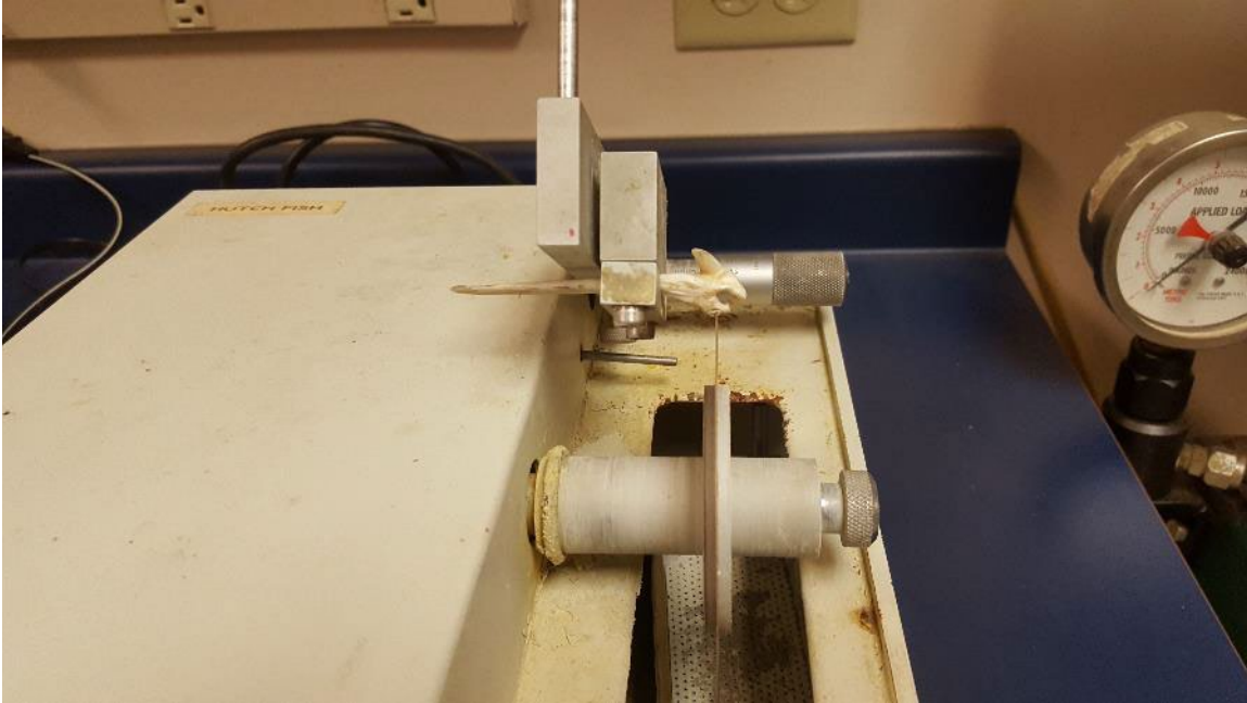
Figure 23. Cutting locations for sectioning catfish pectoral spines. The first cut is at the base of the ventral process with subsequent cuts made distally, 0.5-1.0 mm apart.
