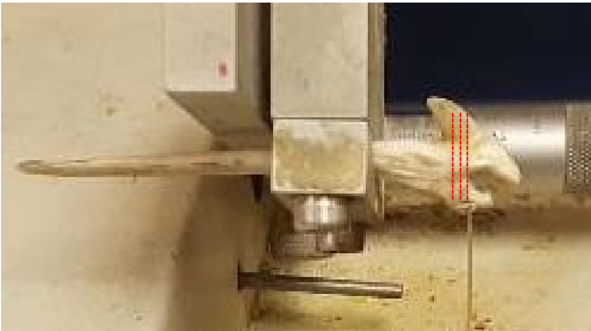
Figure 23. Cutting locations for sectioning catfish pectoral spines. The first cut is at the base of the ventral process with subsequent cuts made distally, 0.5-1.0 mm apart.
