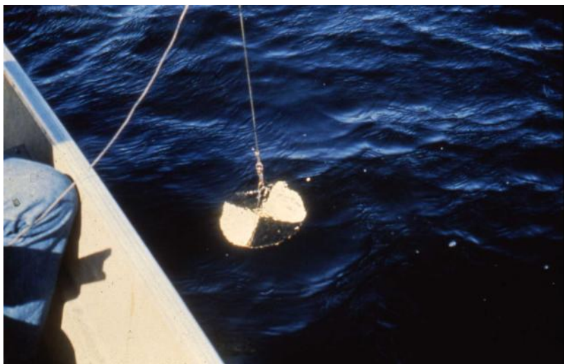
Figure 1. Measuring Secchi Disk transparency.
