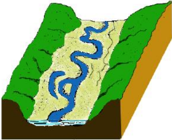
FIGURE 2-2. A broad alluvial valley with gentle gradient showing a meandering stream channel. Scouring and deepening on outside bends form habitat for fish, with riffles between bends providing habitat for juvenile fish and invertebrates.
