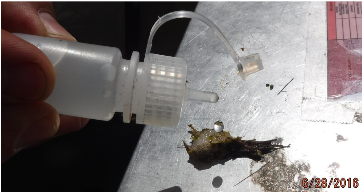
Figure 3. Acid test example reaction and documentation. Tufa sample tested on 6/28/2016 at Tilden 28 Fen, Polk County, MN.
