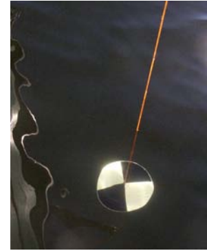
Figure 3. Measuring Secchi Disc transparency
