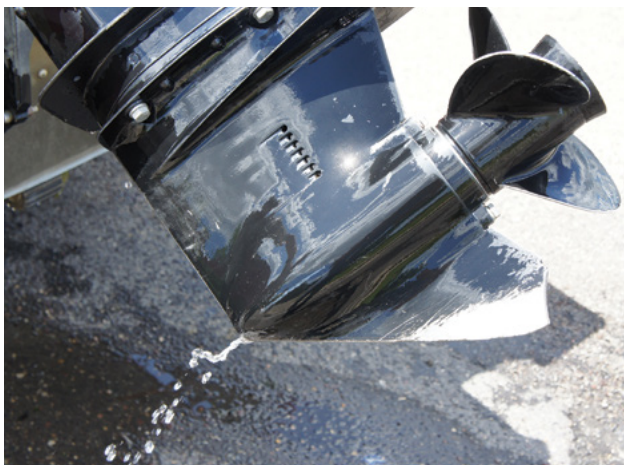
Water draining from a lower unit
