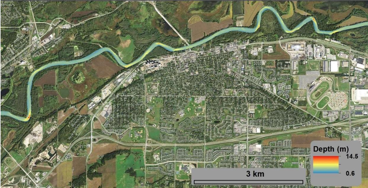
**Figure 7.** Water depth (meters) model from our bathymetric survey of the reach through downtown Chaska and Shakopee (sites I and J in Figure 1) in 2015. Flow is from left to right.
