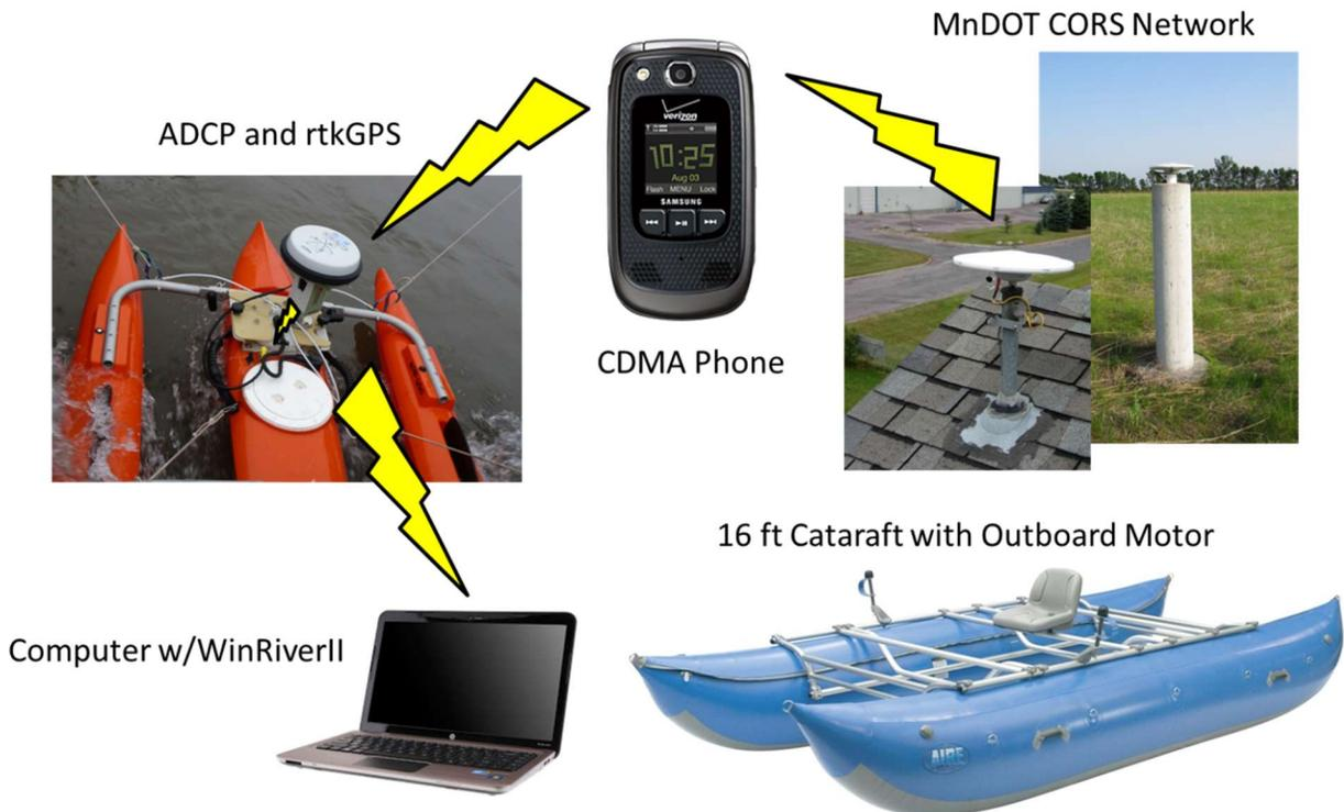
**Figure 2.** Equipment and instrumentation used for bathymetry mapping.
