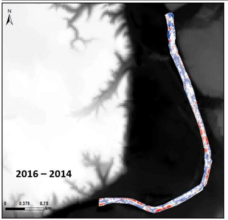
**Figure 9.** DEMs of difference at site D, Mankato, between 2013 and 2014 (top) and 2014 and 2016 (bottom). Erosion is red, deposition is blue, and change below a 25 cm minimum level of change is white.
