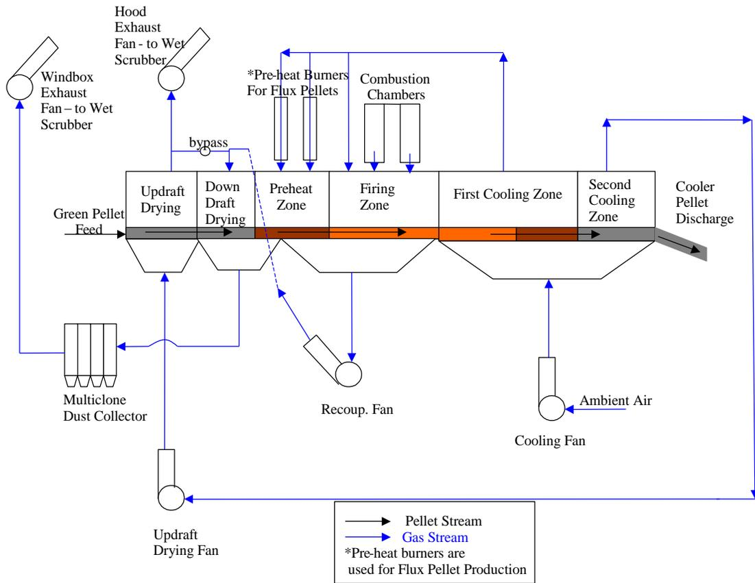
**Figure 2.** Diagram of a straight-grate taconite induration furnace. Fresh pellets are carried on a grate through a furnace and cooled by fresh air passed through the pellet bed. The air used for cooling the hot pellets and the gases generated in the firing zone are used for drying and heating the pellets.
