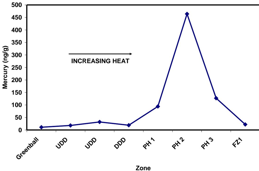
**Figure 4.** Mercury concentrations in dust samples collected from Straight-Grate #1. Concentrations increased to 464 ng/g in the preheat zone and then decreased again as the firing zone was approached.
