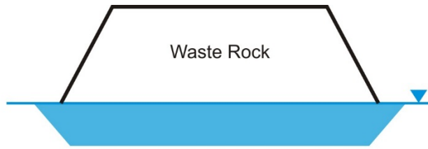
STOCKPILE FOUNDATION MATERIAL BELOW THE WATER TABLE
