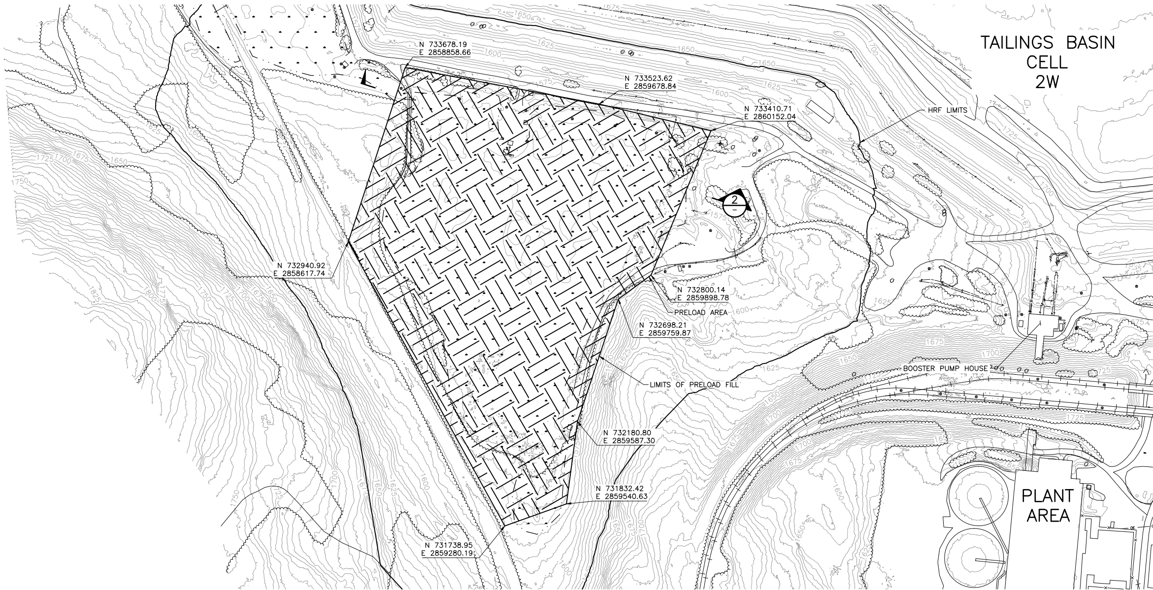
1 PLAN: PRELOAD LAYOUT
