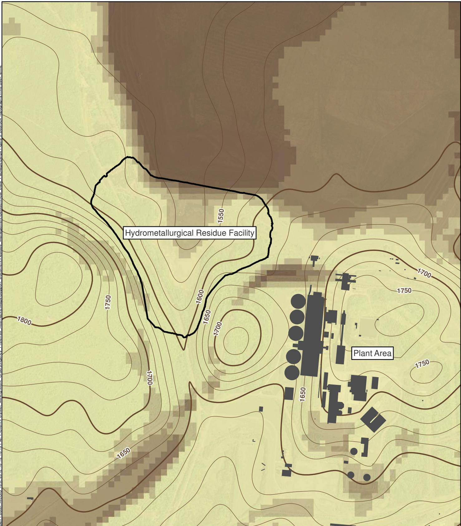
Depth to Bedrock Top of Bedrock (interval = 25 ft)
