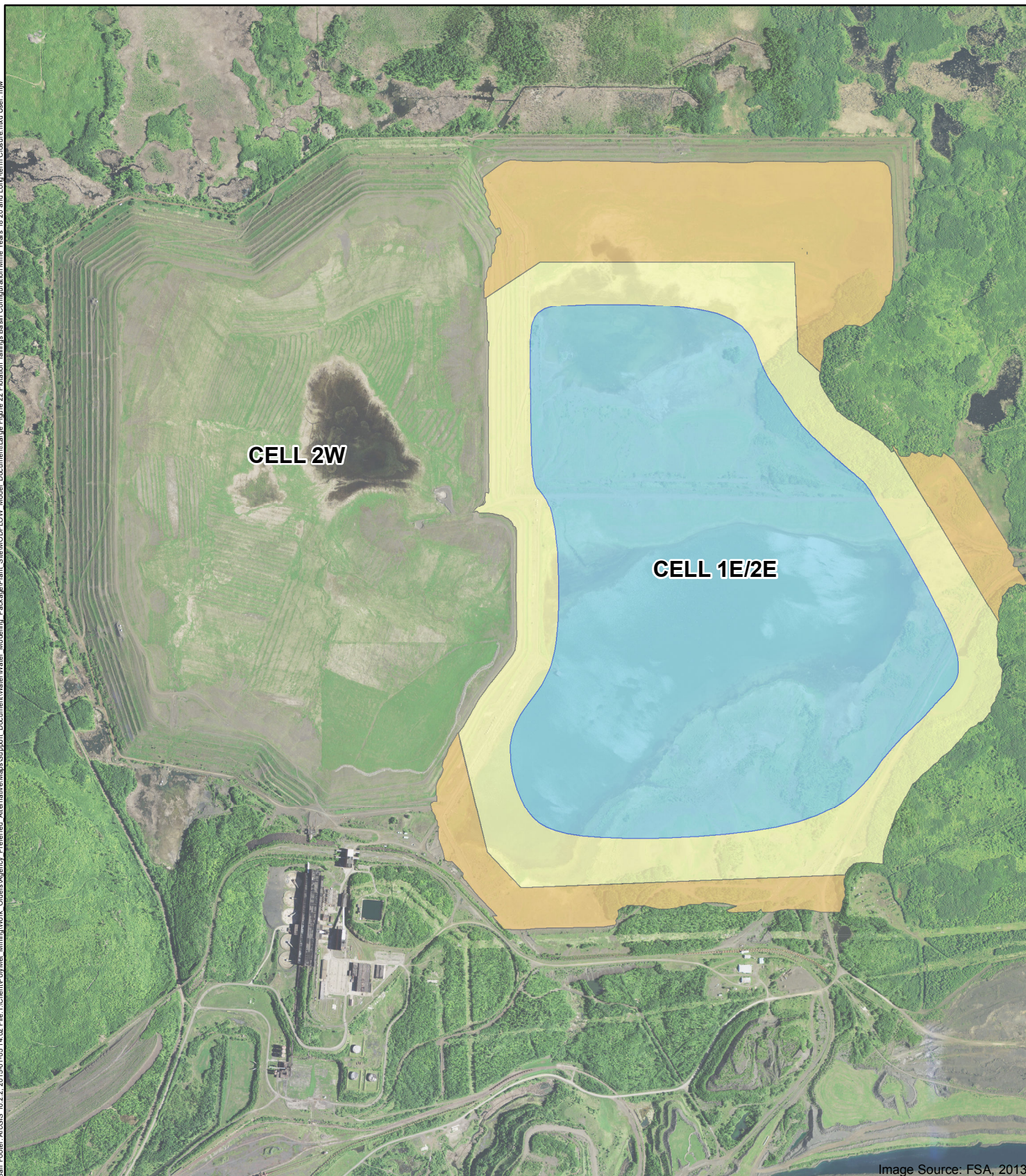
Large Figure 22 FLOTATION TAILINGS BASIN CONFIGURATION - MINE YEARS 18, 20 AND LONG-TERM CLOSURE NorthMet Project Poly Met Mining, Inc.
