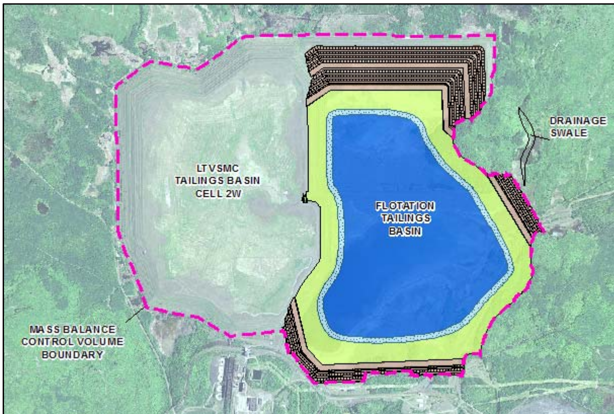
Figure 6-14 Control Volume Boundary for the Tailings Basin Mass Balance
