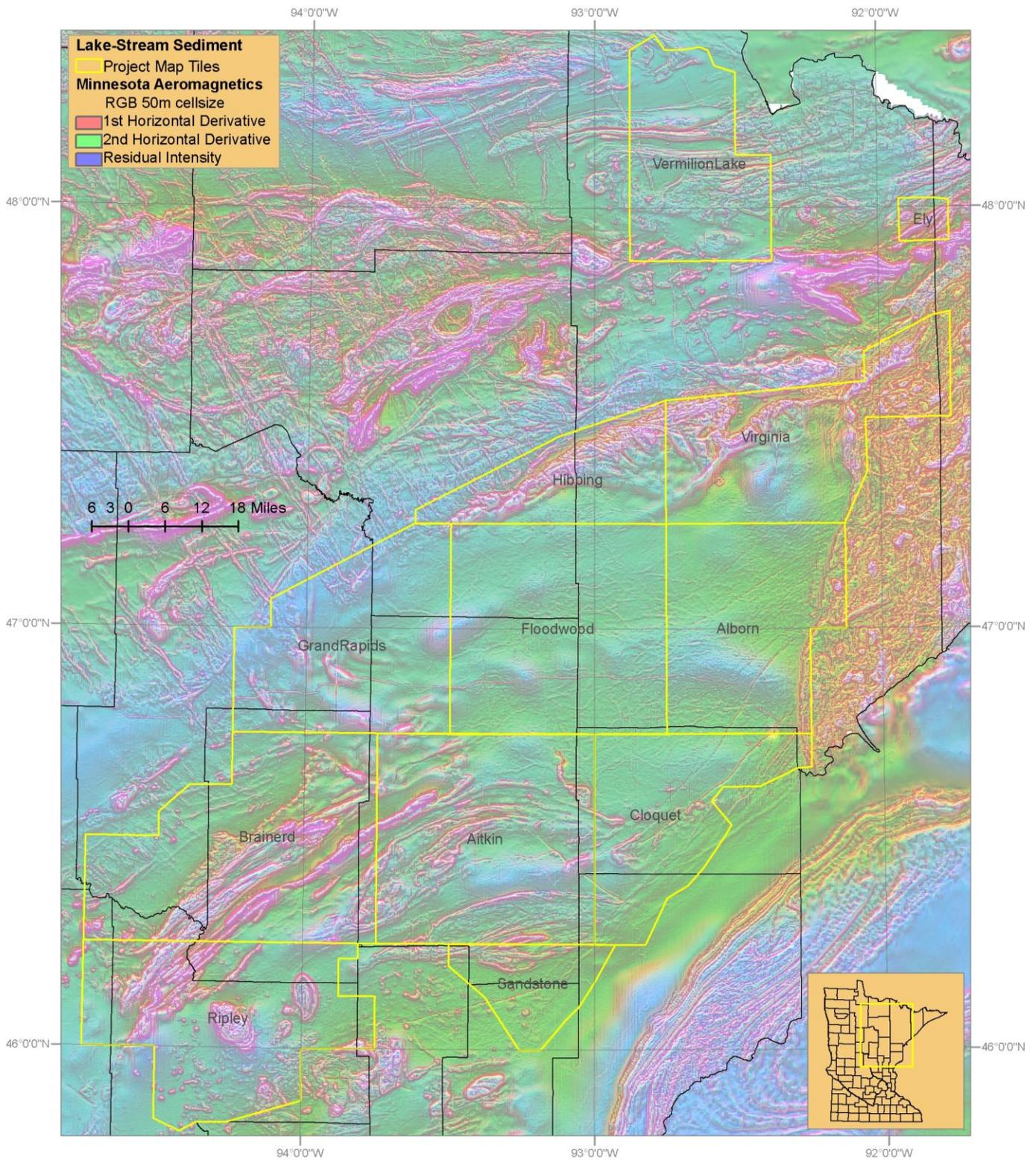
**Figure 13.** Map tiles superimposed on image of Minnesota aeromagnetic data (1<sup>st</sup> and 2<sup>nd</sup> Horizontal derivatives and residual intensity as RGB).
