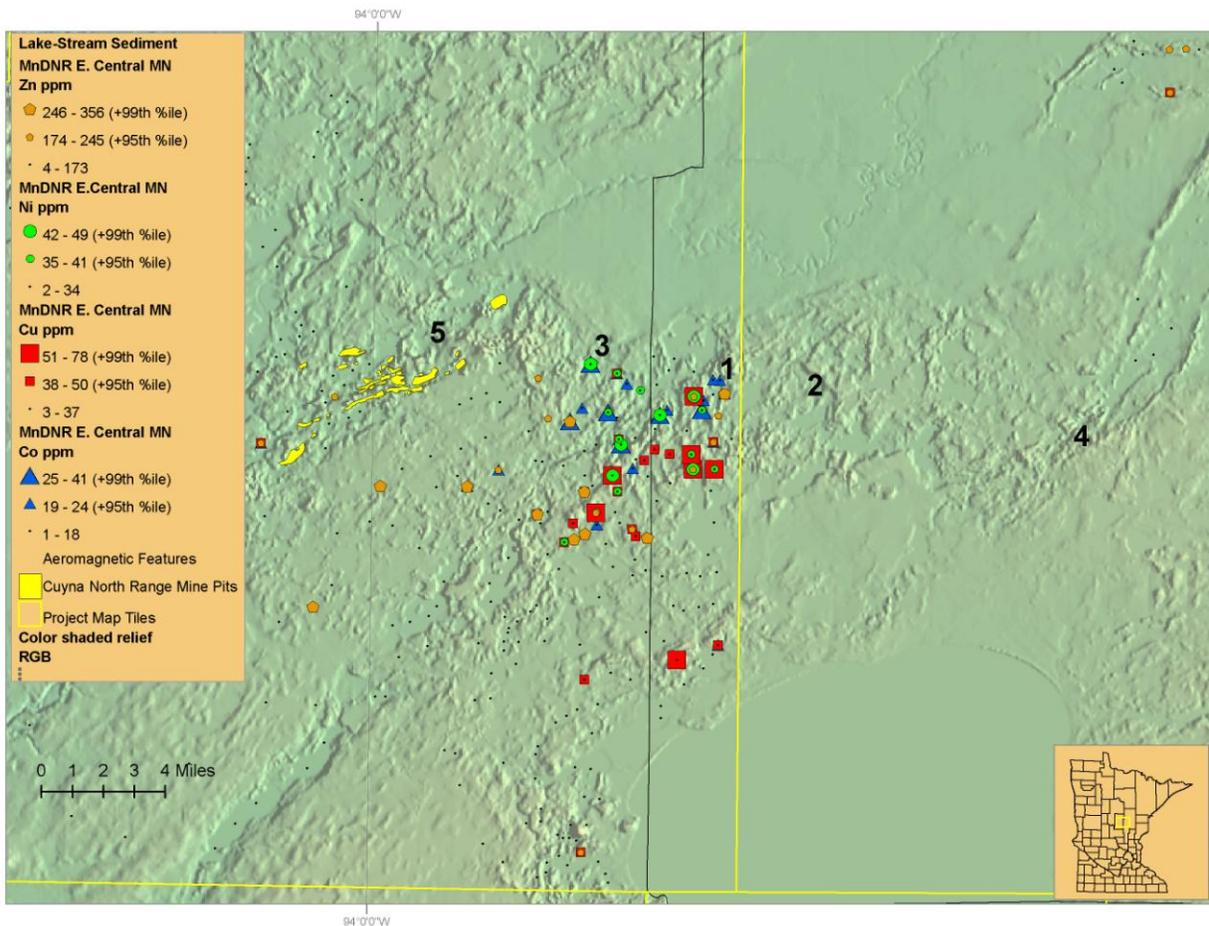
**Figure 22.** Composite Cu-Ni-Zn-Co lake and stream sediment data covering the Deerwood-Aitkin area. Background image of statewide color shaded relief (illumination from the east). Numbered locations discussed in text.
