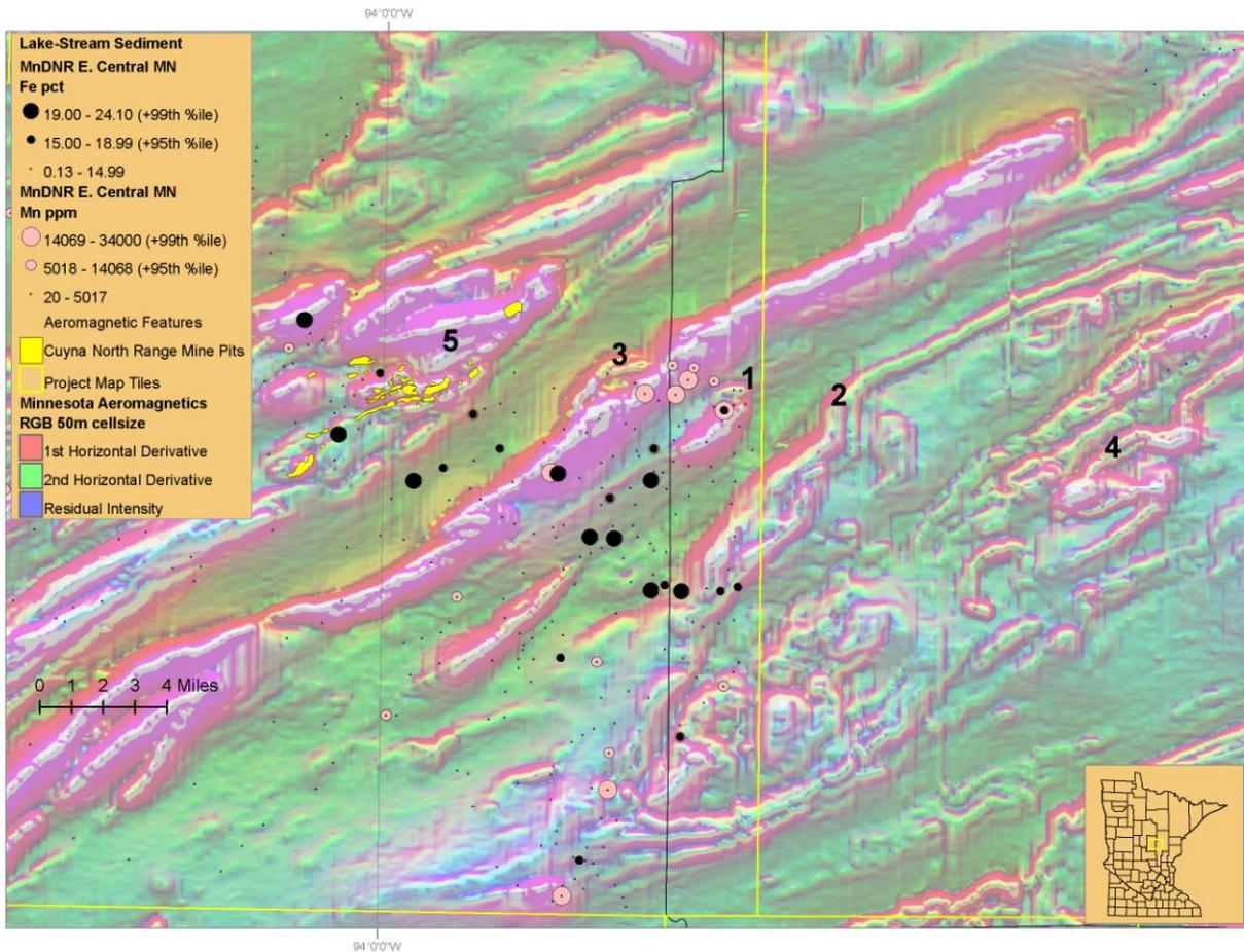
**Figure 25.** Iron values in percent and manganese values in ppm showing +99<sup>th</sup> and +95<sup>th</sup> percentile lake sediment values for MnDNR project 236 area, aeromagnetic background. Numbered locations discussed in text.
