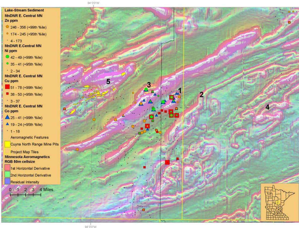
**Figure 23.** Composite Cu-Ni-Zn-Co lake and stream sediment data covering the Deerwood-Aitkin area. Background image of statewide aeromagnetic data (1<sup>st</sup> and 2<sup>nd</sup> horizontal derivatives and residual magnetic intensity as an RGB image). Numbered locations discussed in text.
