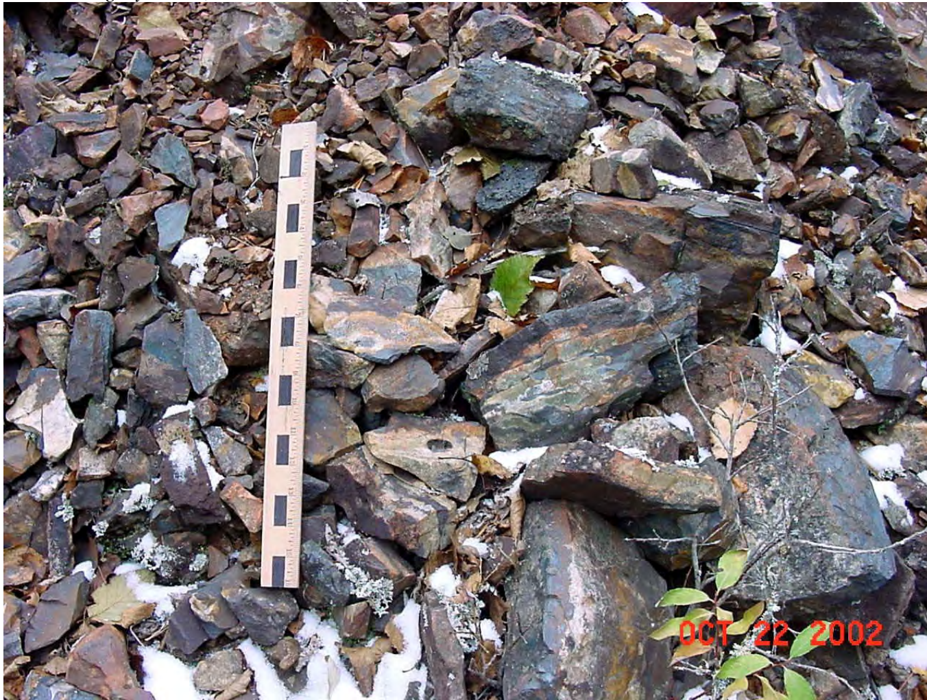
Photo 162f, stockpile 113, Taconite (Natural Ore). Ruler scale—each black bar is 1 inch long.
