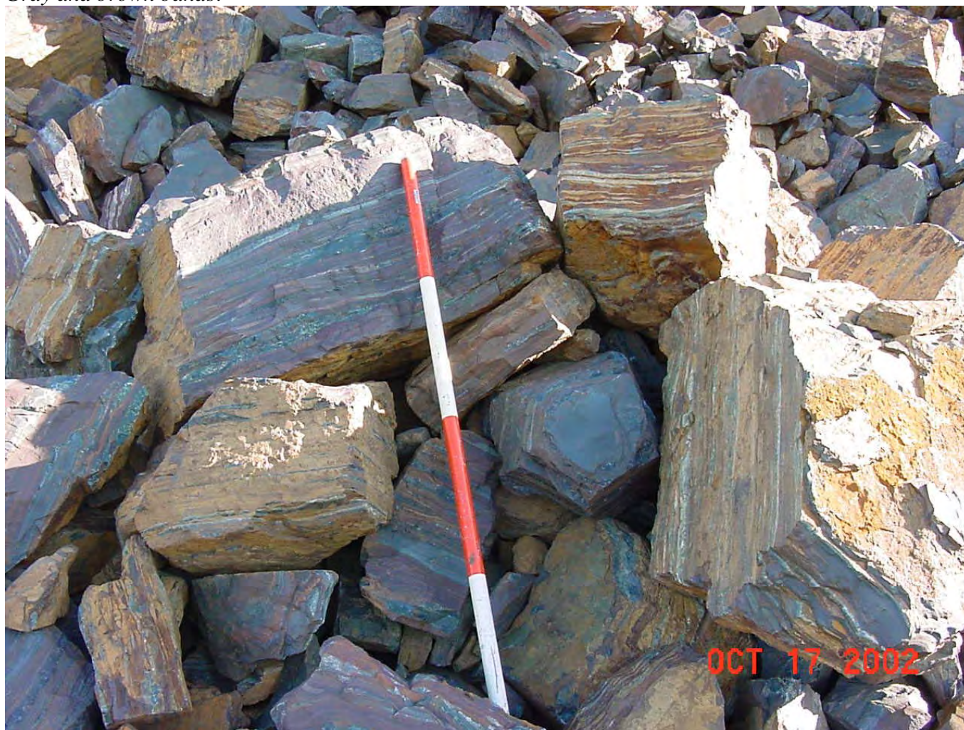
Photo 145f, stockpile 7010, lean taconite. Red and white rod—each band is 1 foot long.
