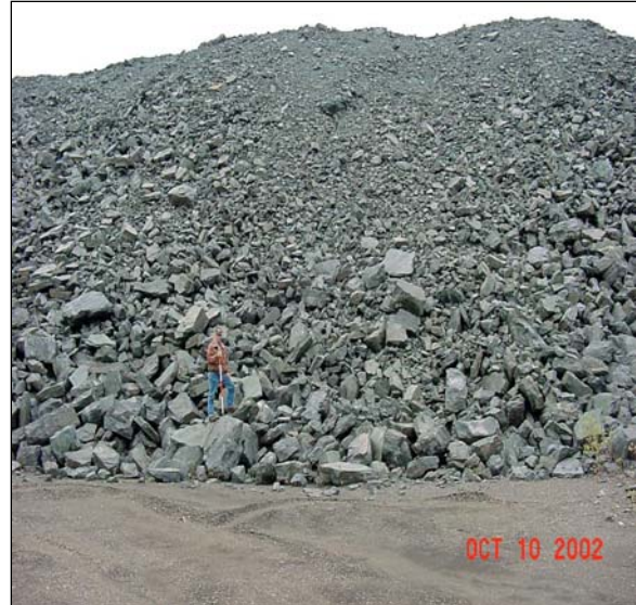
Figure 8. Most stockpiles are accessible to the toe of at least one lift. Often access is available from the top of the lift.
