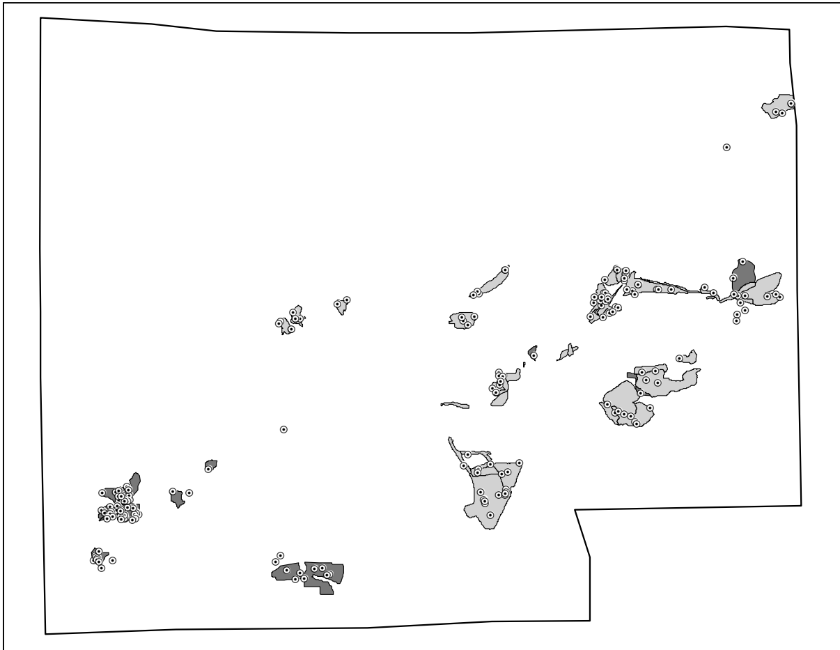
Figure 5. Map of field sites (small circles with dots) associated with mine stockpiles and other mining features. The light gray areas represent rock stockpiles and the dark gray areas represent overburden stockpiles.
