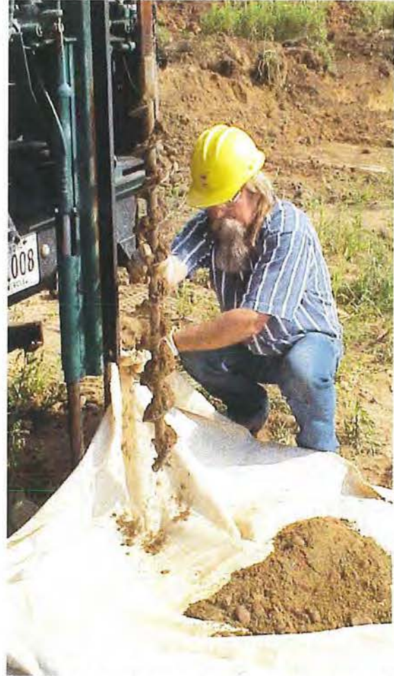
Figure 8. Collecting all material on mat and later splitting the sample with 1/4 method.
