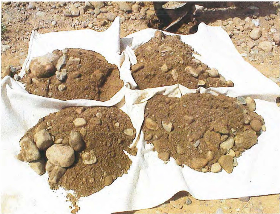
Figure 13. Splitting the sample in quarters using the shovel handle method.
