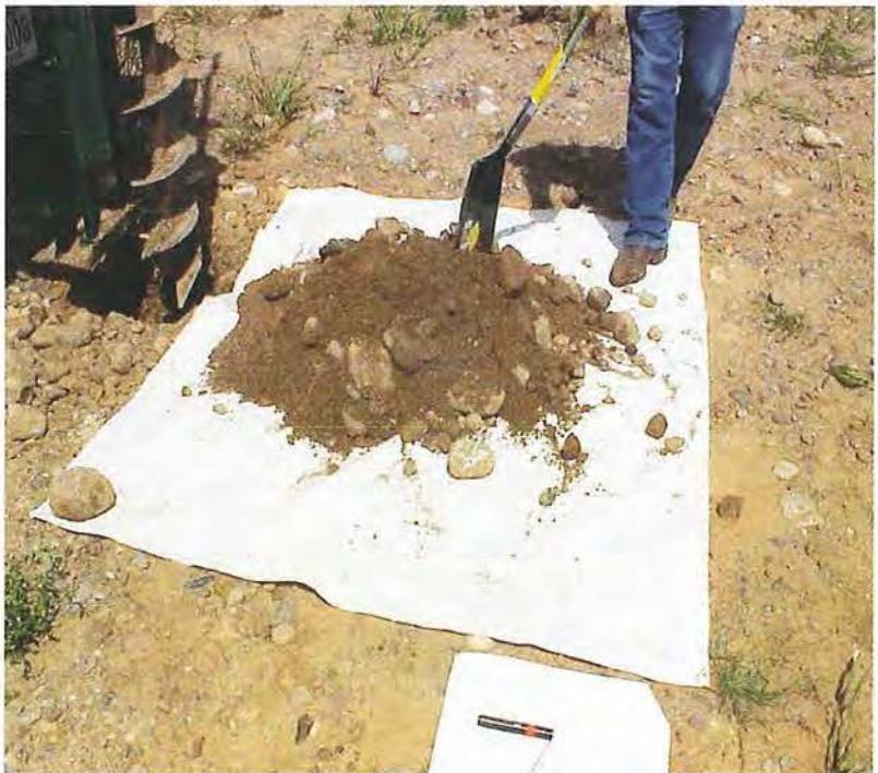
Figure 11. Quartering the sample using the shovel method.
