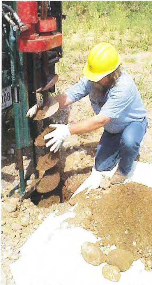
Figure 7. Random sampling technique-sampling 1 in every 3 or 4 auger flights.
