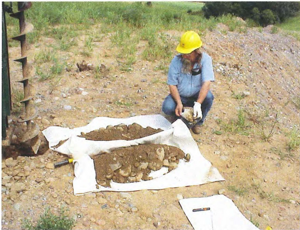
Figure 12. Splitting the sample in half using the shovel handle method.
