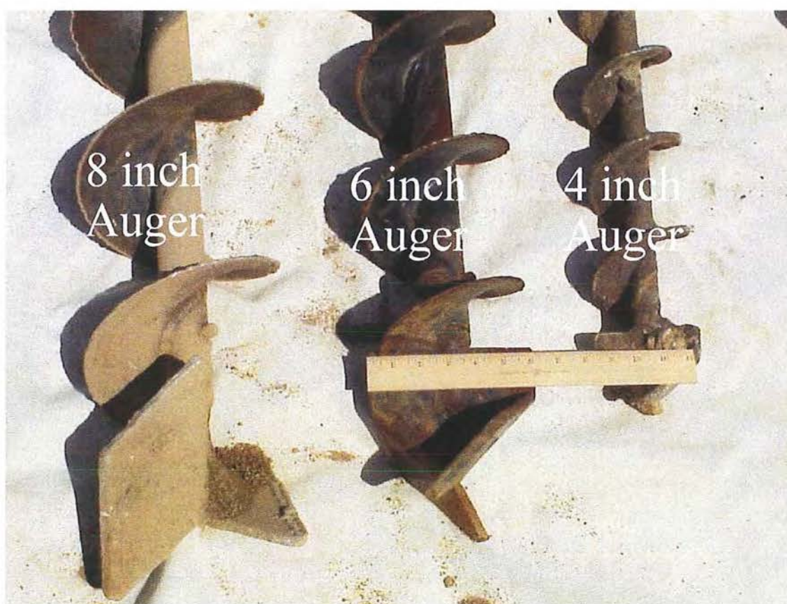
Figure 6. Different diameter augers used for drilling sand and gravel (top). The 8 inch, 6 inch, and 4 inch auger used in this study (bottom).
