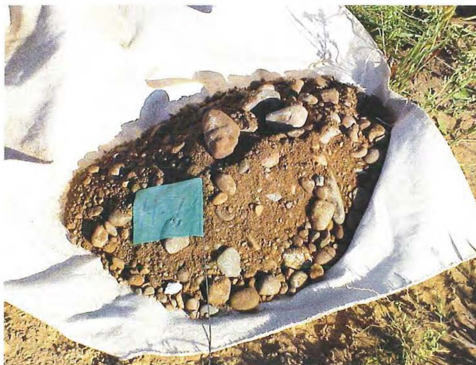
Figure 21. Material collected from the 6-inch auger drilling. Material collected only from the auger (top). Material collected only from the mound (bottom). Note the auger material is much finer than the material collected from the mound.
