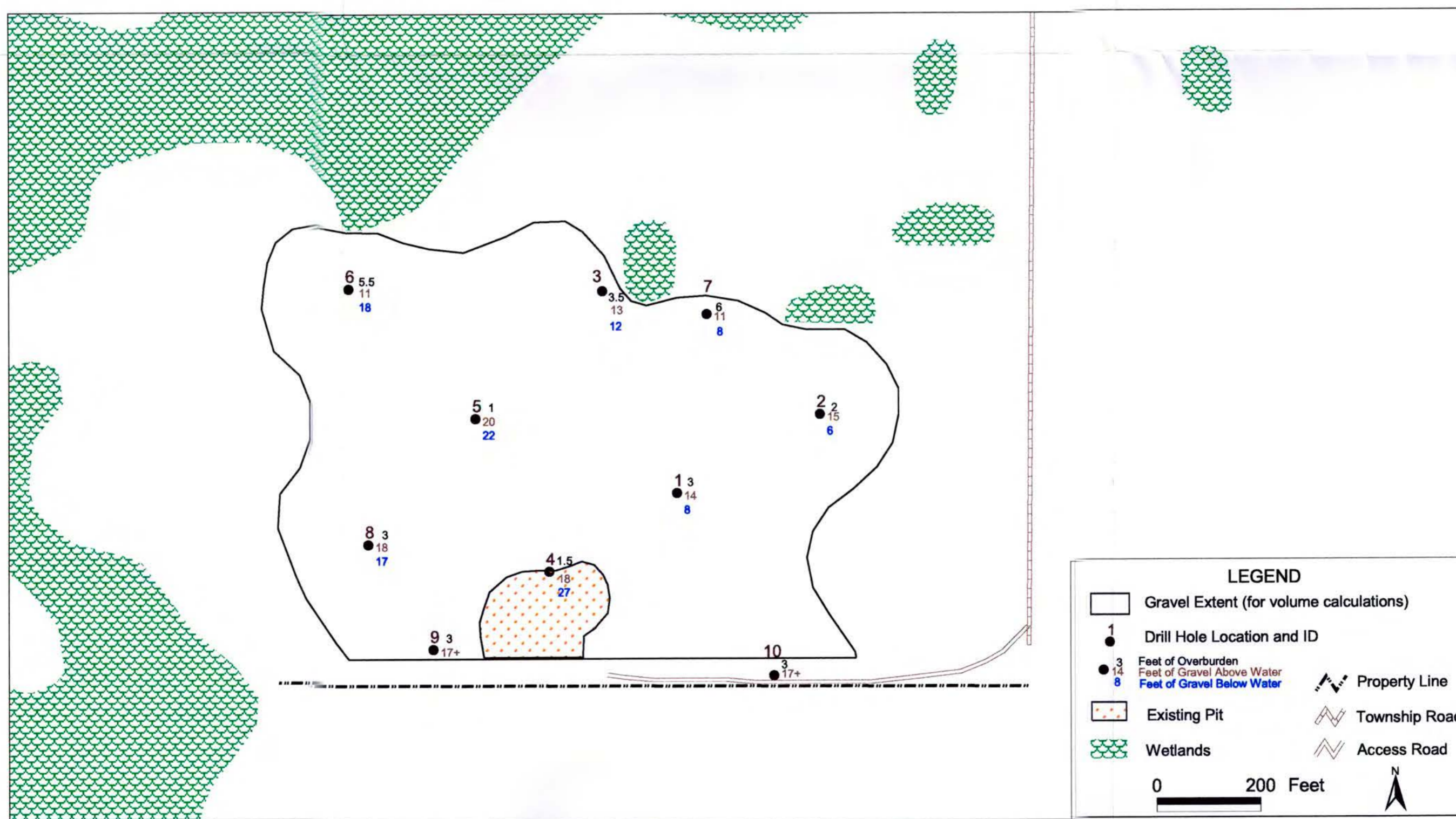
Feet of overburden, feet of gravel above and below the water table, and wetlands from the National Wetlands Inventory are displayed above. The gravel is thinner and the water table is slightly more shallow in the northeast as compared to the southwest. The overburden is generally thicker in the northern holes. Holes 9 and 10 were stopped prior to drilling through the gravel.
