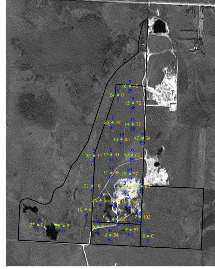
Deposit thickness (in feet) above water table Drill hole ID and location — 18 • 82 — Deposit thickness (in feet) Deposit thickness (in feet) below water table
