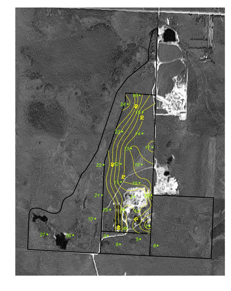
18 • Rotosonic drill hole - ID and location Deposit thickness (10 foot contours)
