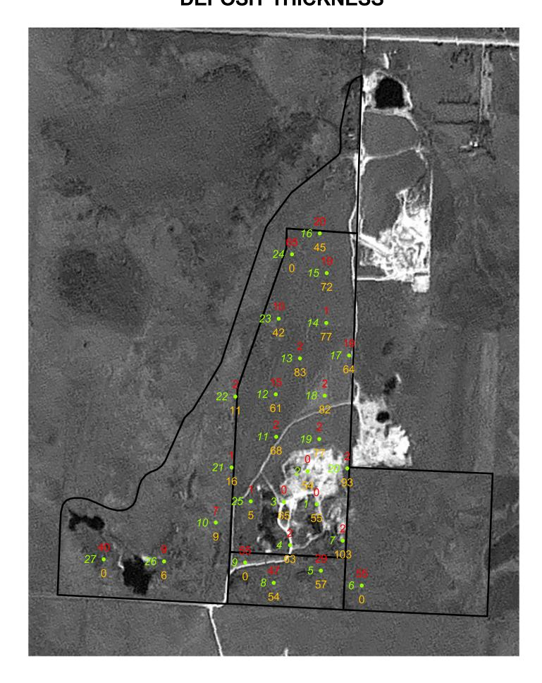
2 — Overburden thickness (in feet) Drill hole ID and location —— 18 • 82 — Deposit thickness (in feet)
