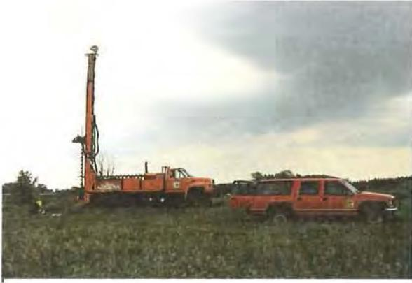
Figure 3. Drilling Rig with a 10 inch diameter, 25 ft continuous flight auger (above).
