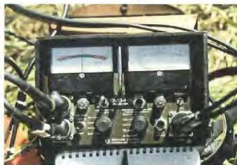
Figure 7. Receiver operator taking EM conductivity readings (left).
