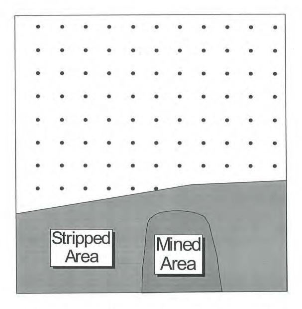
Figure 10. Location of EM Conductivity stations. Eight lines were completed (east-west), seven of the lines contained 11 stations each and the last line contained six stations, totaling 83 stations.
