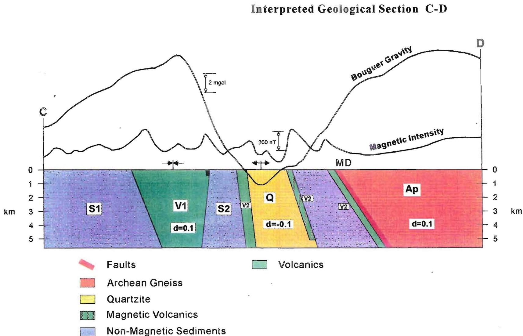
Figure 13. Camp Ripley Area. Gravity profile is observed data, magnetic profile is a modeled qualitative correlation modified from Spector (1995).
