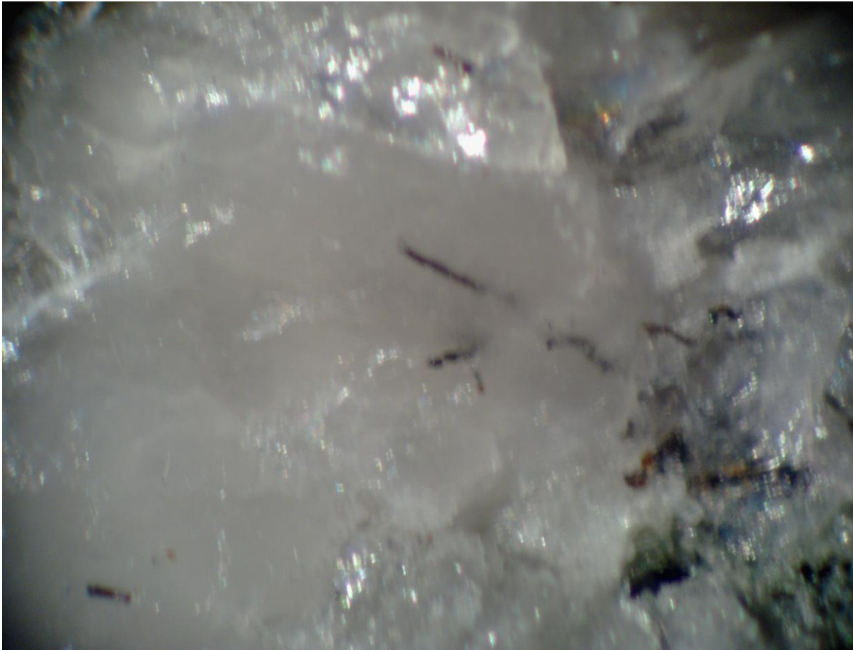
Figure 4. From DDH R-11 at 80.9'; shows typical rutile needles. Horizontal field of view is about 3 mm.
