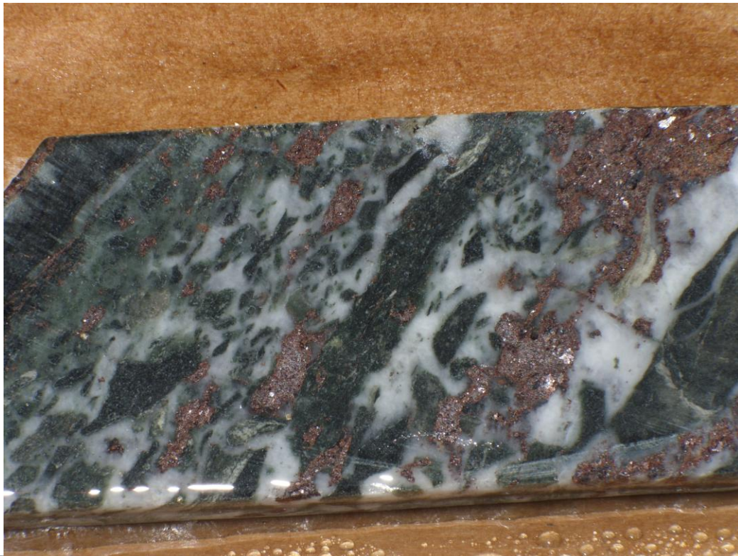
Figure 33. DDH SXL-4 @143.45' showing brecciated chloritic volcanics, sphalerite, and quartz. Sphalerite filling voids(?).
