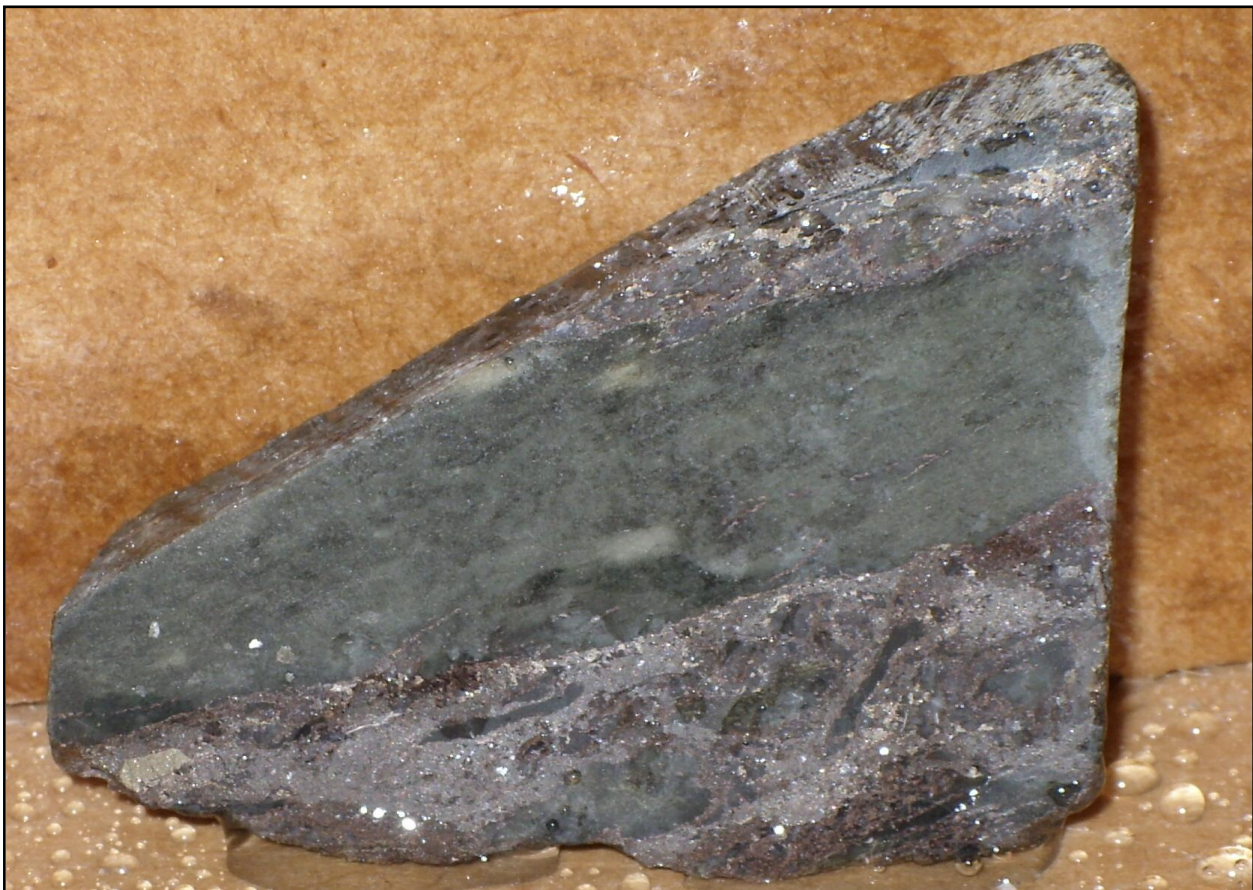
Figure 31. Comparison of gold-bearing and non-gold-bearing sphalerite and brecciated chert, felsic volcanics, or quartz vein(?). Rock is wet. Vertical sample dimension is 3.6 cm.
