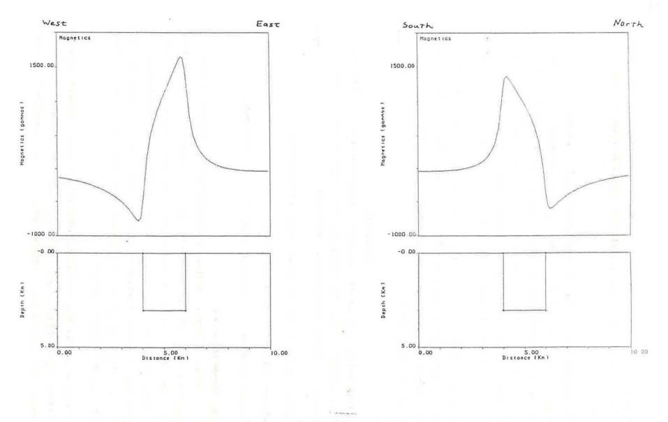
Figure 2. Magnetic anomalies along (a) west-east and (b) southnorth profiles, over a vertical prism that has a strong remanent magnetization (inc.,dec. = 40<sup>0</sup>,290<sup>0</sup>).
