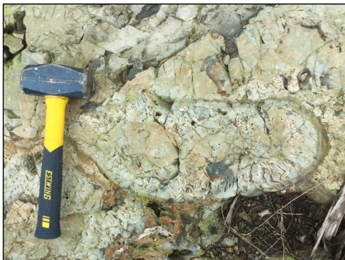
Figure 11: Strongly epidotized and silicified pillowed basalt at station 18DL-LR020 in southwest Ran. In a VMS environment, sulfide deposits typically form stratigraphically above epidote and silica alteration zones.
