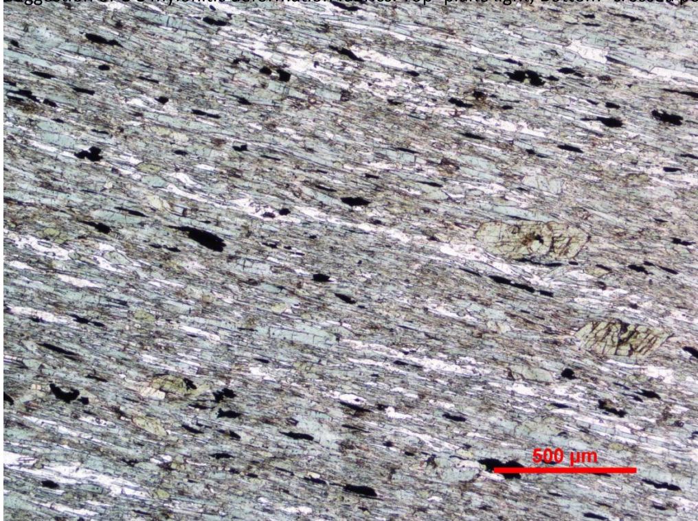
Sample CR-0026. Mylonitic amphibolite with gneissic quartz-plagioclase segregation lenses. Note suggestion of C-S mylonitic deformation fabrics. Top- plane light; Bottom- crossed polarizers.
