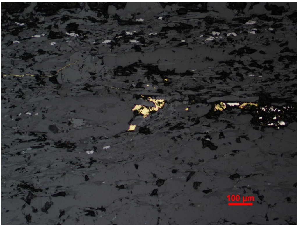
Sample CR-0026. Disseminated chalcopyrite associated with disseminated epidote in quartz-plagioclase segregation lens. Top- plane light; Middle- crossed polarizers; Bottom- reflected light.
