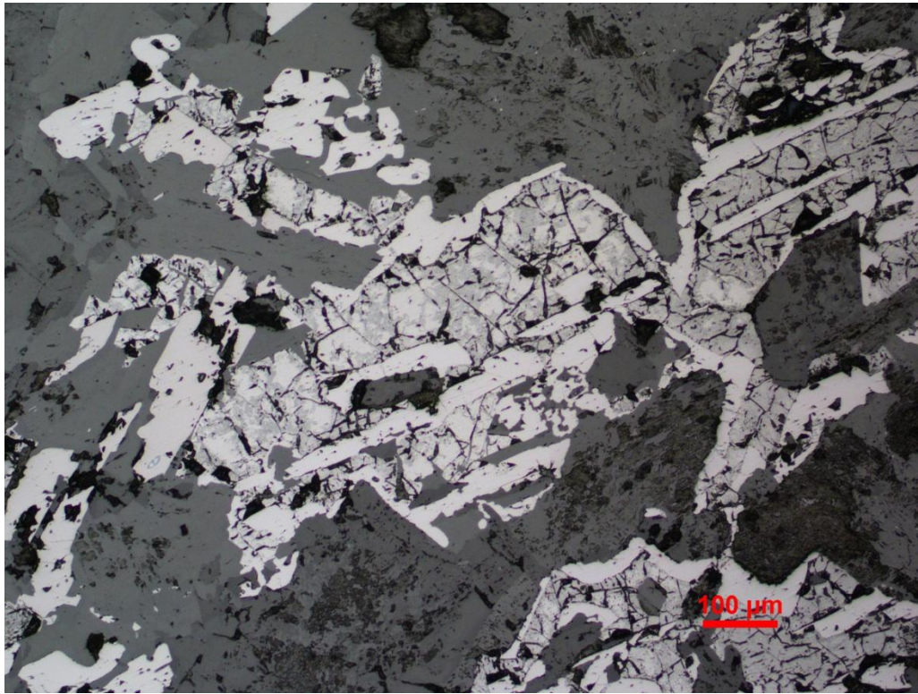
Sample CR-0005. Close-up view of magnetite with exsolved ilmenite. Magnetite is locally replaced by titanomagnetite(?). Reflected light.
