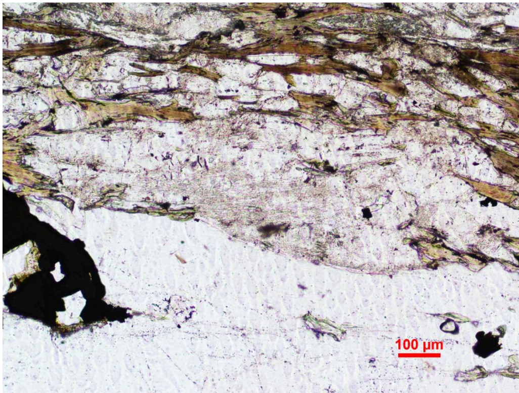
Sample CR-0002. Subhedral staurolite microporphyroblasts and disseminated ilmenite in foliated biotite schist. Top- plane light; Middle- crossed polarizers; Bottom- reflected light.
