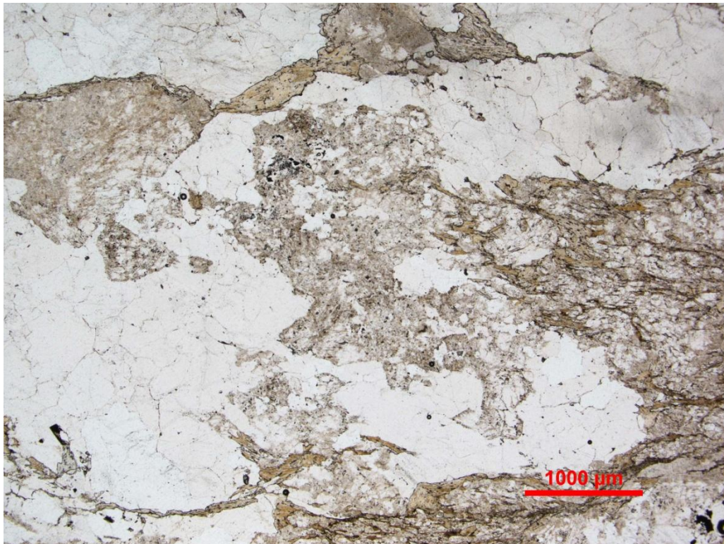
Sample CR-0002. Albitic twinning in anhedronal plagioclase in thin segregation band of coarser grained quartz-plagioclase-biotite. Note pale green chlorite locally replaces biotite. Top- plane light; Bottom- crossed polarizers.
