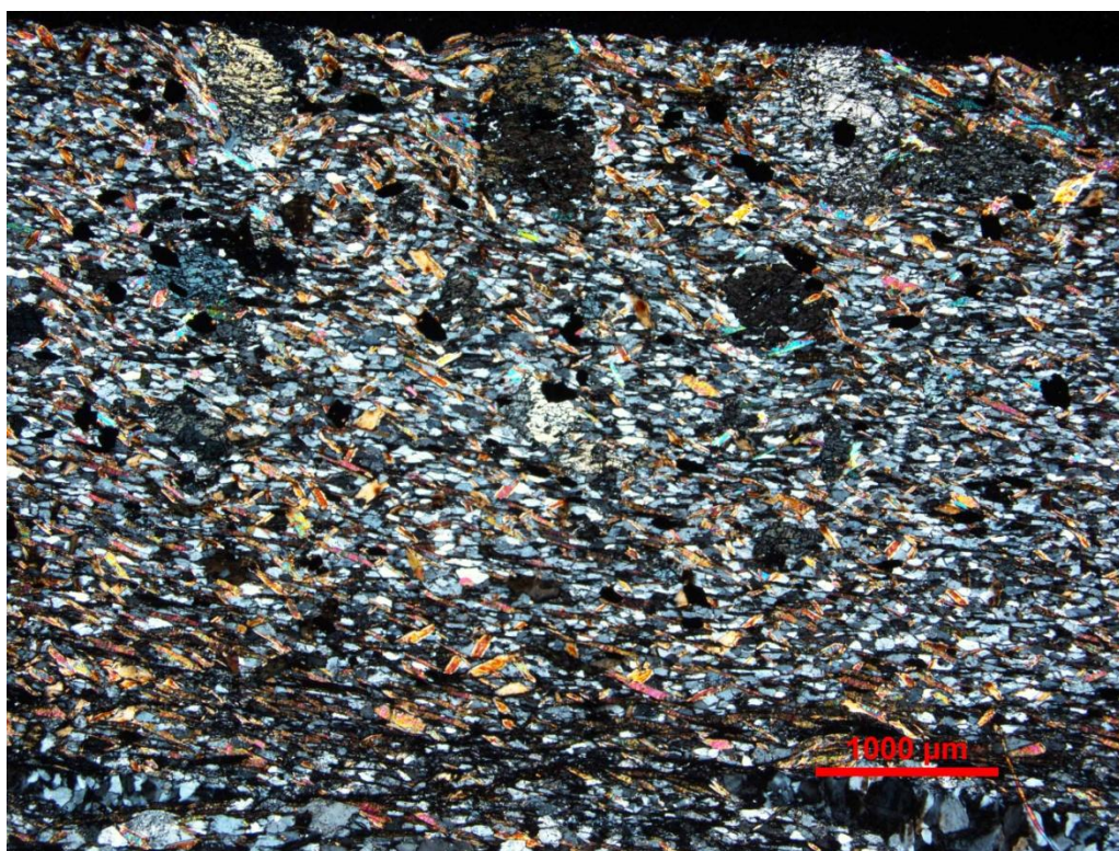
Sample CR-0002. Subhedral staurolite microporphyroblasts (across top) in gneissic, mylonitic schist. Top- plane light; Bottom- crossed polarizers.
