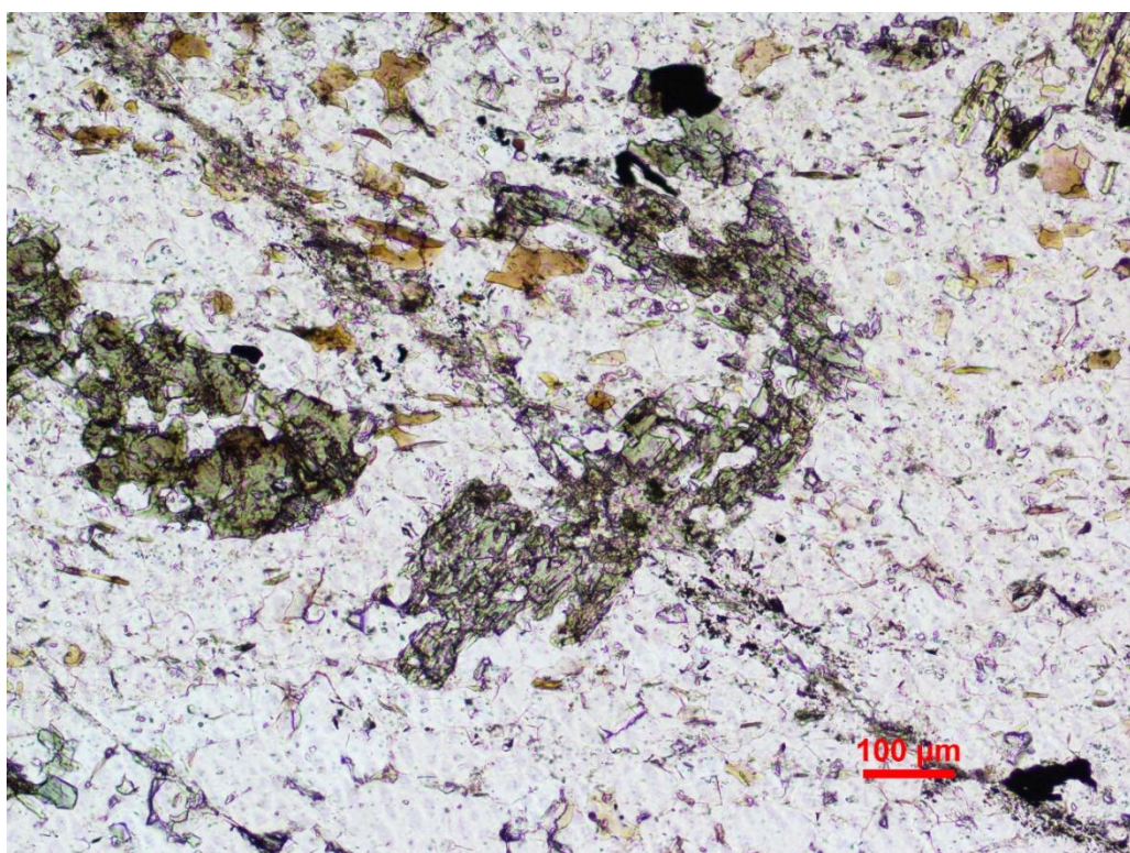
Sample CR-0001. Disseminated, elongated chlorite grain parallels chlorite veinlet, both perpendicular to biotite foliation. Plane light.
