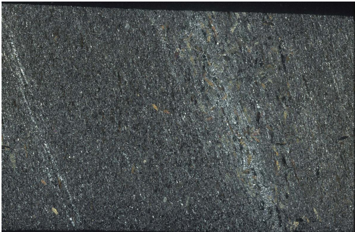
Sample CR-0001. Wide-field, full thinsection view showing very fine grained biotite phyllite/schist with localized amphibole porphyroblasts. Note suggestion of incipient gneissic banding. Top- plane light; Bottom- crossed polarizers.
