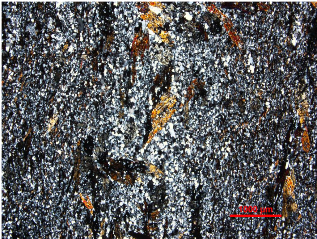
Sample CR-0001. Relict(?) fold forms in amphibole porphyroblasts. Top- plane light; Bottom- crossed polarizers.
