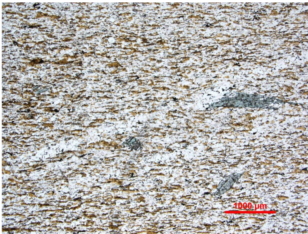
Sample CR-0001. Biotite foliation superimposed across quartz veinlet. Plane light.
