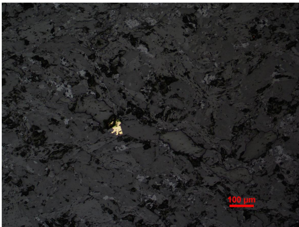
Sample CR-0021. Chalcopyrite associated with irregular carbonate veinlet. Top- plane light; Middle- crossed polarizers; Bottom- reflected light.
