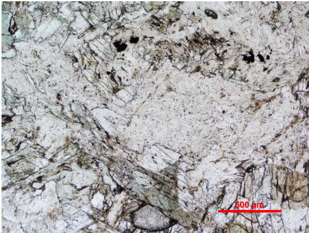
Sample CR-0006. Remnants of brown-green pleochroic magmatic hornblende with overgrowths and replacements by colorless, metamorphic amphibole. Note colorless amphibole partly replaced by chlorite. Top- plane light; Bottom- crossed polarizers.
