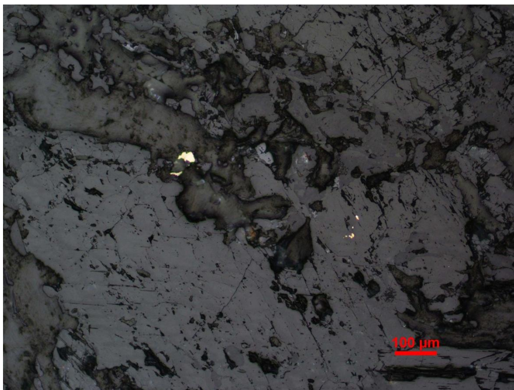
Sample CR-0006. Fine, subhedral-anhedral, disseminated chalcopyrite associated with chlorite, calcite and amphibole. Top- plane light; Middle- crossed polarizers; Bottom- reflected light.
