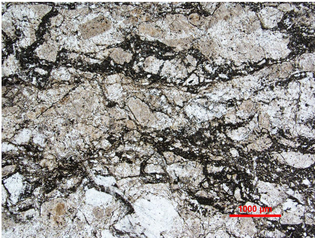
Sample CR-0004. Accessory zircon inclusion in plagioclase (center), metamorphic green biotite (lower right), and weak sericite alteration. Top- plane light; Bottom- crossed polarizers.
