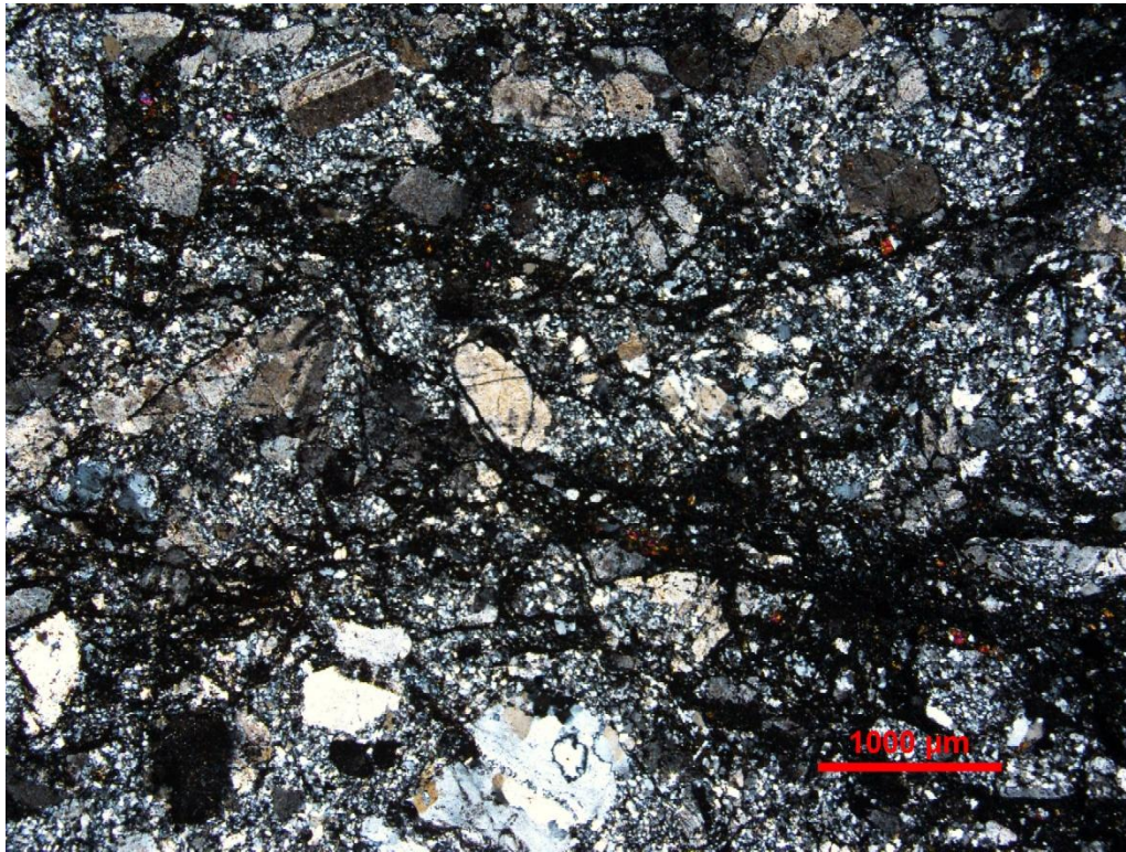
Sample CR-0004. Brittle fault breccia with fine epidote breccia matrix. Top- plane light; Bottom- crossed polarizers.
