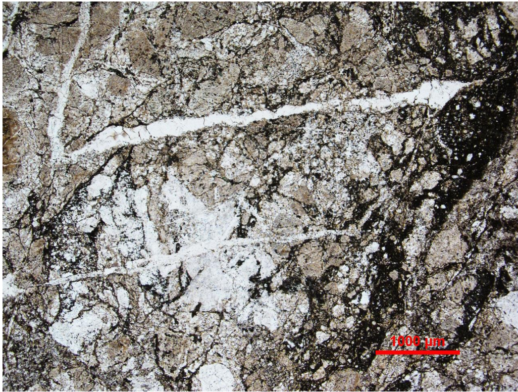
Sample CR-0004. Quartz veins cutting fault breccia and truncated by late fault (at right). Plane light.
