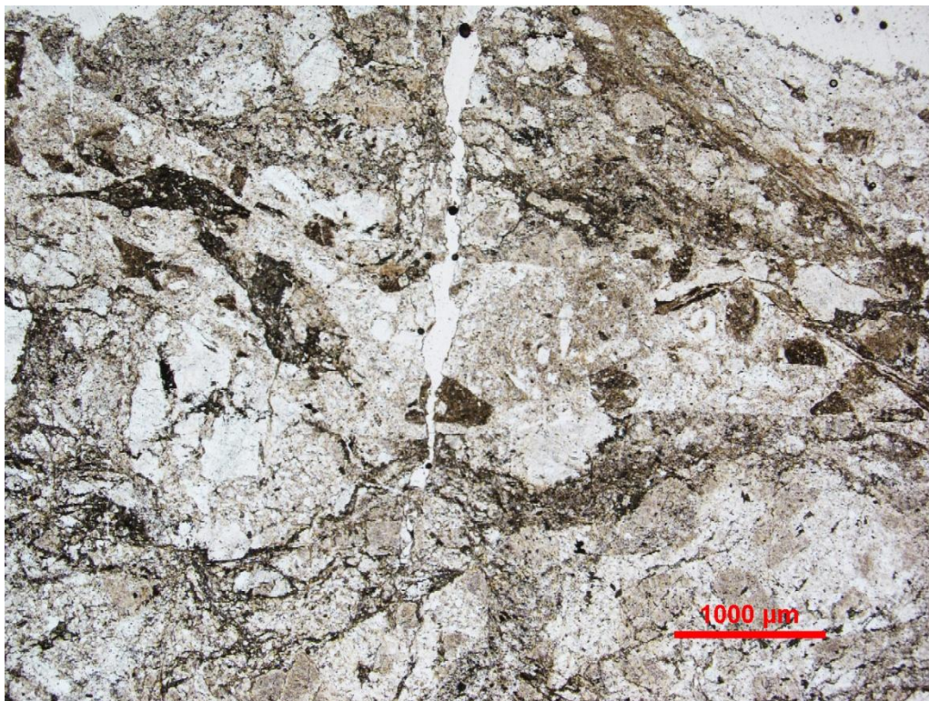
Sample CR-0004. Angular re-brecciated fault breccia fragments in fault breccia. Plane light.
