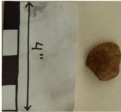
Figure 22: A pebble representative of the gossan lithological category. Pebble has been left dry to better show color. Each block on the scale card is one inch long.
