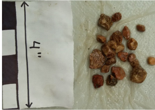
Figure 18: A handful of pebbles representative of the coarse-grained pink granite lithological category. Pebbles have been spritzed with water to better show color and textures. Each block on the scale card is one inch long.
