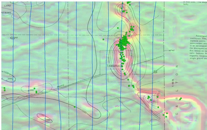
Figure 7. The Tamarack Intrusive Complex area in east-central Minnesota showing 1948 USGS flight line traces and magnetic contours superimposed on 3-band imagery of MGS 2nd-generation data, and recent drill hole locations (green dots).
