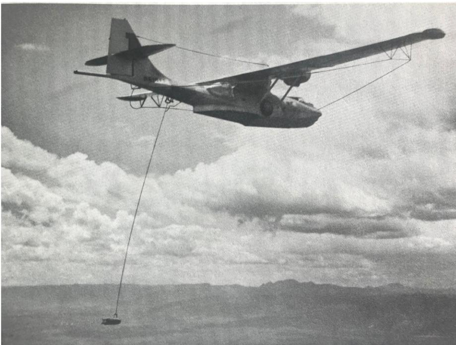
Figure 2. INPUT Mark V airborne electromagnetic survey platform in use. Image from Barringer (1965). Super Canso (PBY Catalina) aircraft with electromagnetic transmitter loop extending to wingtips, towed receiver "bird", and aft-mounted "stinger magnetometer".
