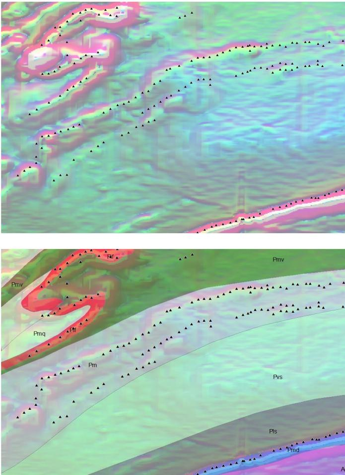
Figure 9 (upper image). Electromagnetic conductor peaks (black points) superimposed on MGS 2nd-generation imagery. Figure 9 (lower image). Same area with MGS map S-21 bedrock geology map units. Conductor point spacing reflects 1/4 mile flight line spacing.
