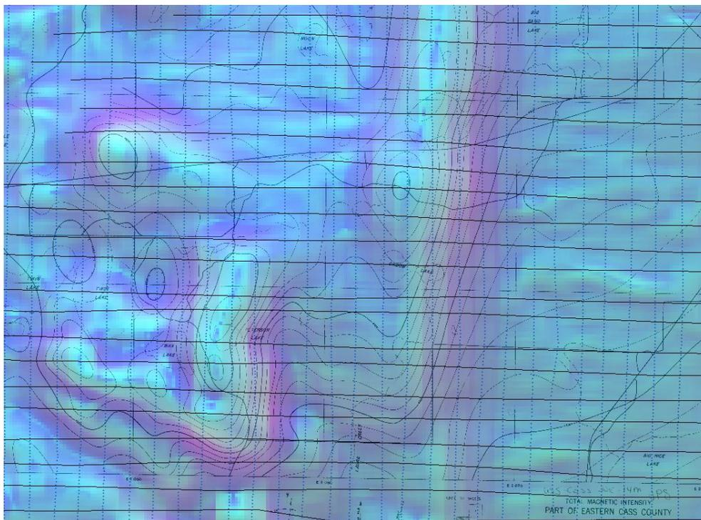
Figure 6. 1951 historical airborne survey data (black contours and east-west flight lines) from a survey between the Cuyuna and Mesabi Iron Ranges, superimposed on 3-band imagery of MGS 2nd-generation data having north-south flight lines.
