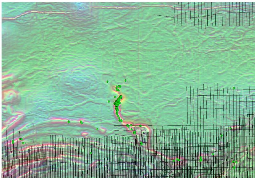
Figure 8. Distribution of historical airborne survey flight lines deployed in sulfur, base metal and uranium exploration near the Tamarack Intrusive Complex. For scale, flight lines are 1/4 or 1/2 mile line spacing.
